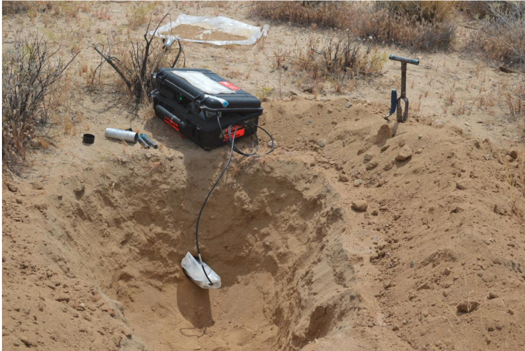
Figure 2: The ambient gamma radiation field within the first burial hole is measured with a sodium iodide gamma spectrometer.
