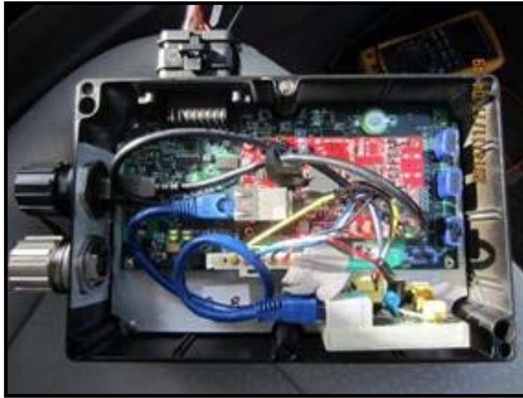
Figure 2. The on-board data collection box was installed in a vehicle and relayed data to the charger when the vehicle was charging.
