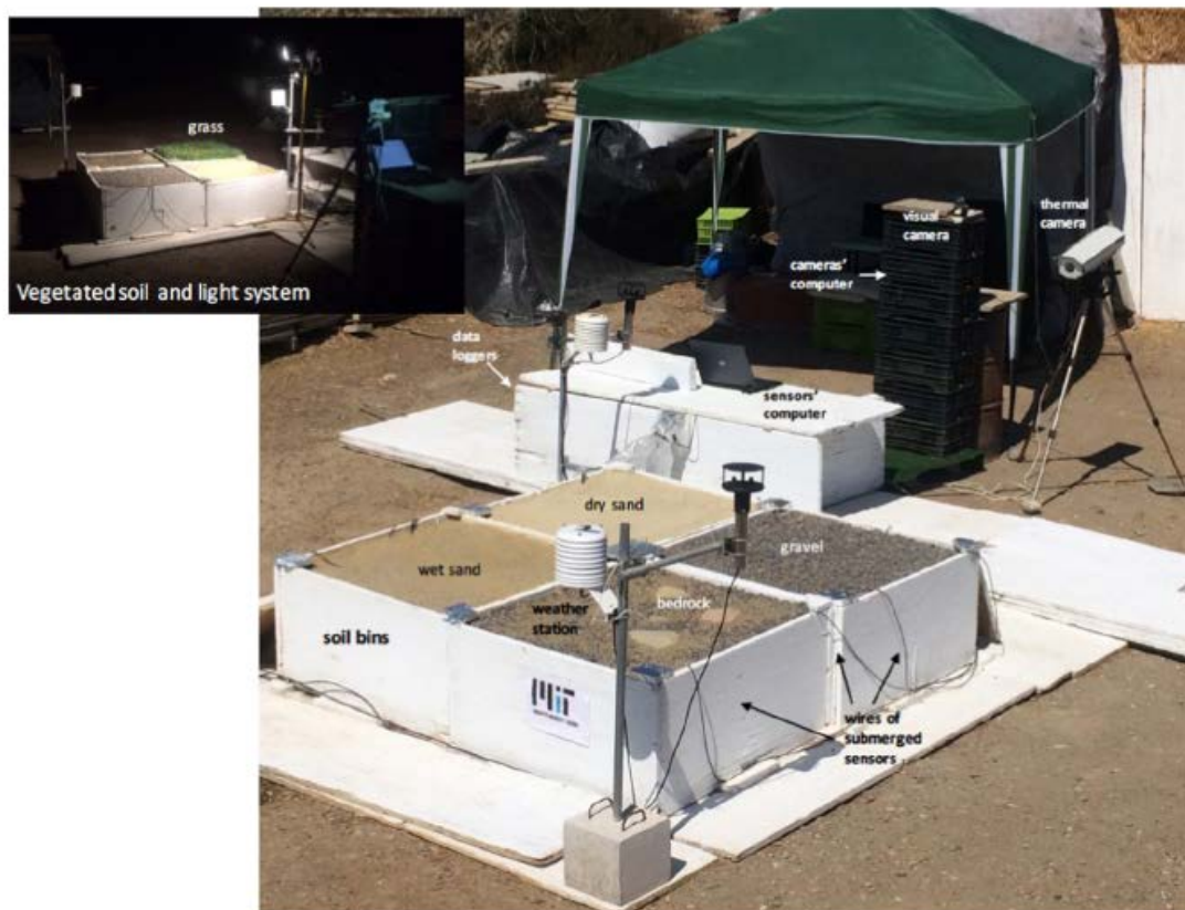
Figure 28. Testing site specifically built for these experiments. Notice the modular and scalable configuration of the soil bins as well as the accessible disposition of the place for setting sensors and hardware. Observe, at the top left corner, the second configuration of this testing site with a soil bin with grass (top right corner) and the artificial lighting system used at night
