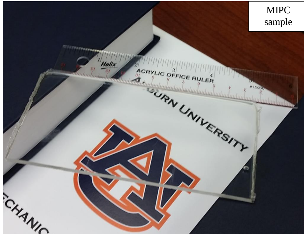
Figure 3. A sample MIPC produced at Auburn University showing excellent optical transparency. The target/logo is located ~50 mm away from the sample plane demonstrating superior optical clarity achieved.
