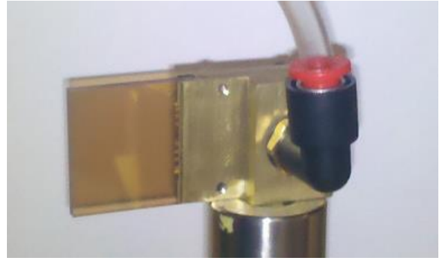
Fig. 112. Schematic and image of the air cooling system with a high absorption VBG attached. Normal VBG's have an absorption of approximately 10^{-4} \text{ cm}^{-1} and are clear. The absorption of this VBG was artificially increased by 140 times to allow for the simulation of 11 kW beams.
