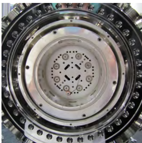
Figure 14: View of the opened vacuum chamber of the phase 2 setup from the bottom. On the outside, one can see the vacuum chamber. The two silver rings on the inside are the two heat shields, which are made of silver-plated copper. The inner shield has a much thicker wall for better magnetic shielding.
