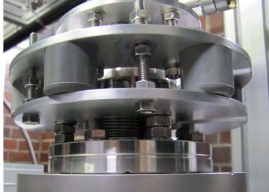
Figure 16: Vibrational decoupling at the vacuum chamber is done with a membrane bellow. The freely shaking coldfinger is resting on top of gray rubber pieces which absorb the vibrations.
