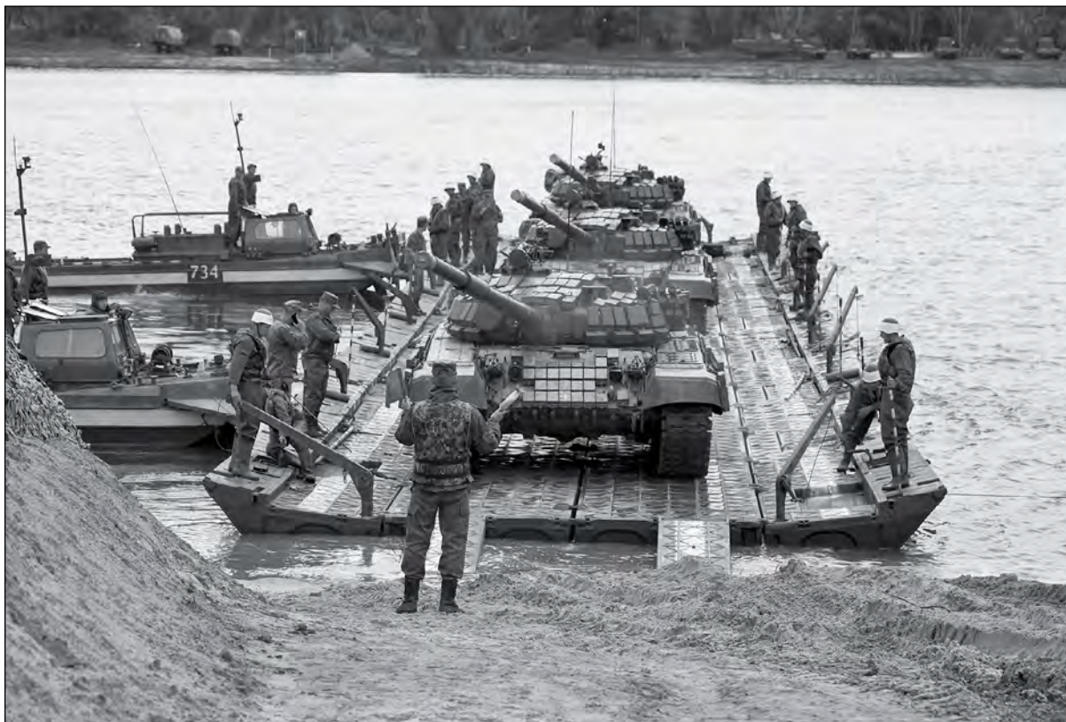
Pontoon bridge system functioning as a ferry
