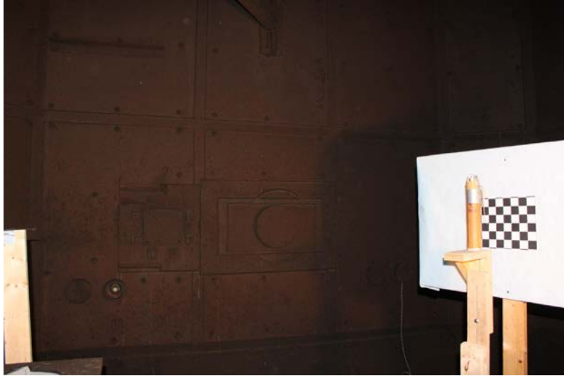
Fig. 31 The TNT charge assembly (minus detonator), positioned on the wooden platform within the ARL small blast chamber (also see Fig. 30). This configuration was used for high-speed imaging of the detonation and explosion.
