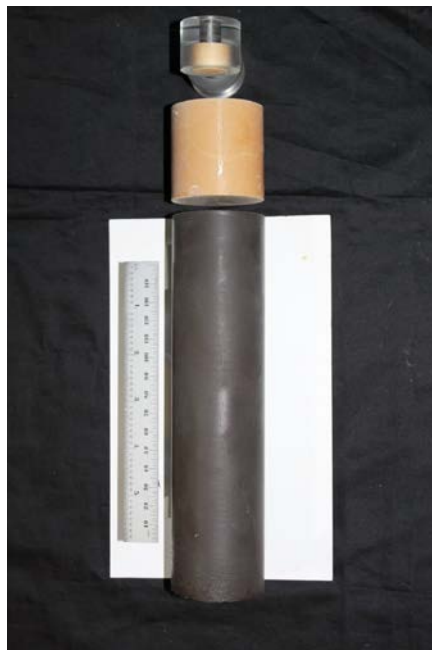
Fig. 28 A photo of the components of the TNT:Mg:B charge used in the tests. The black color of the main charge is caused by the B additive.
