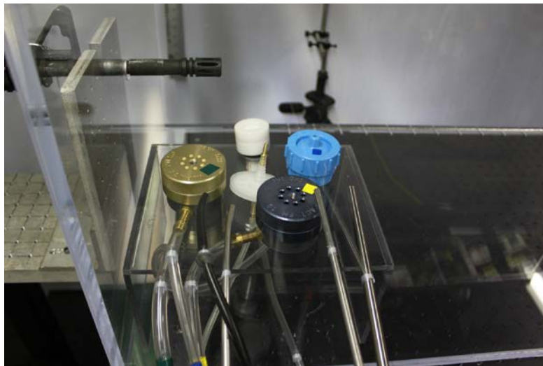
Fig. 6 The particle and gas samplers within the PMMA enclosure. Note the proximity to the “birdcage”.
