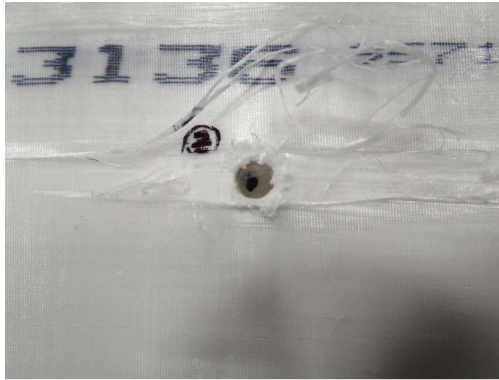
Fig. 8 Indentation site shown from top, showing portion of top plies (with permanent marker dot) that has been plugged and remains at the bottom of the indentation hole after testing
