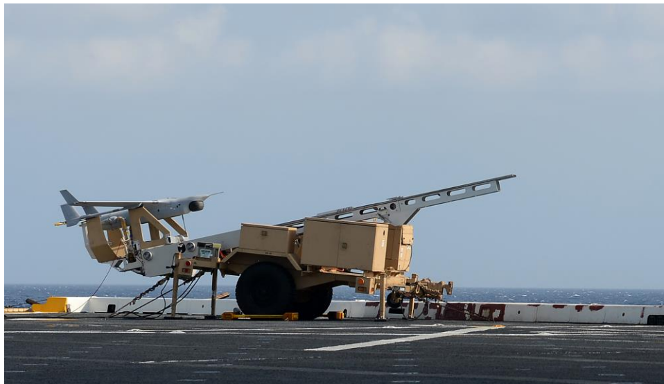
Figure G-5 RQ-21A Blackjack and Launcher on the flight deck of USS Mesa Verde
