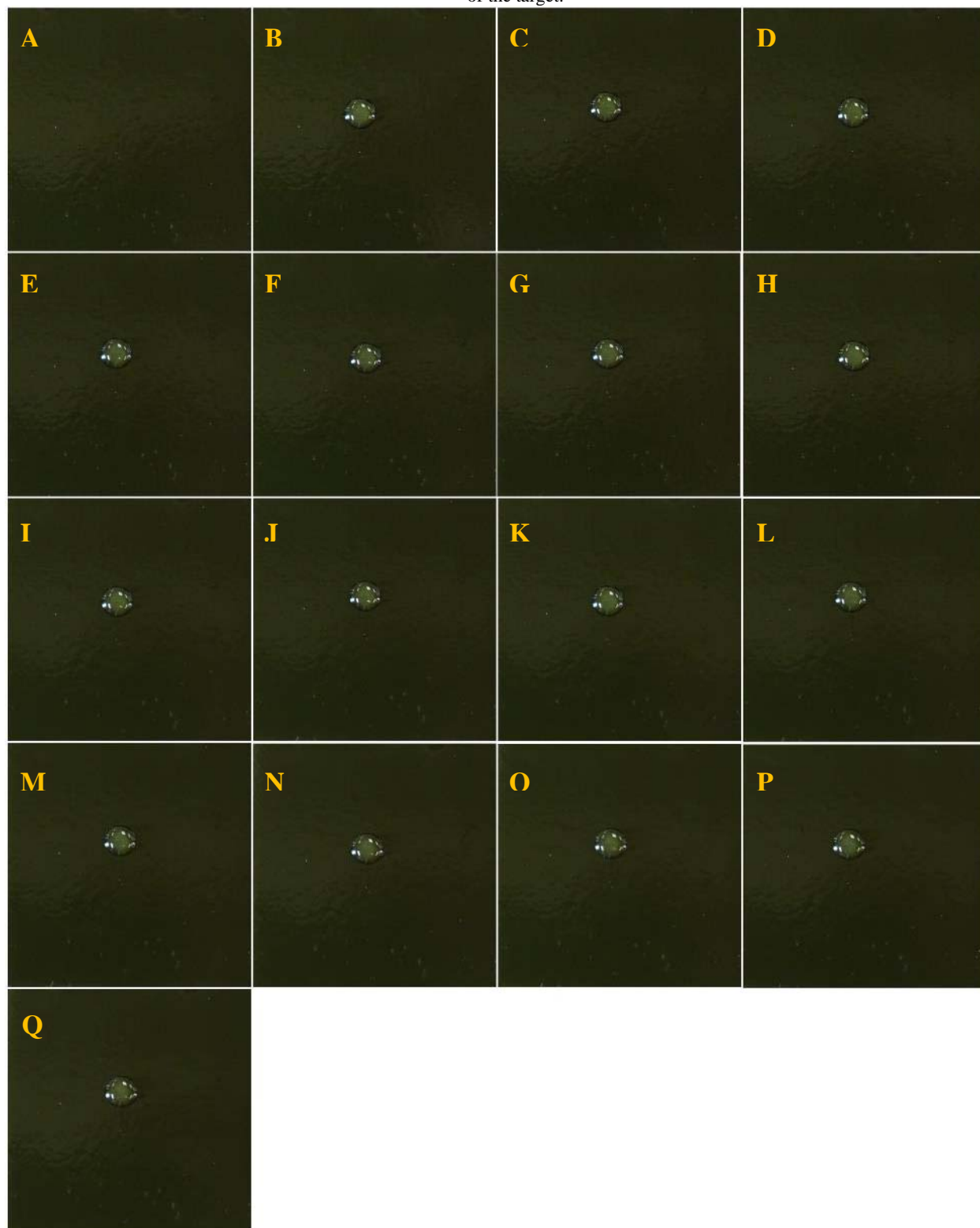
Fig. D2 — MES on the PDMS-polyurethane coating. Images of a coupon before application (A) and at 0 (B), 0.5 (C), 1 (D), 1.5 (E), 2 (F), 2.5 (G), 3 (H), 3.5 (I), 4 (J), 4.5 (K), 5 (L), 10 (M), 15 (N), 20 (O), 25 (P), and 30 (Q) min following application of the target.
