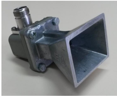
Fig. 6.21. Rectangular horn feed antenna.
