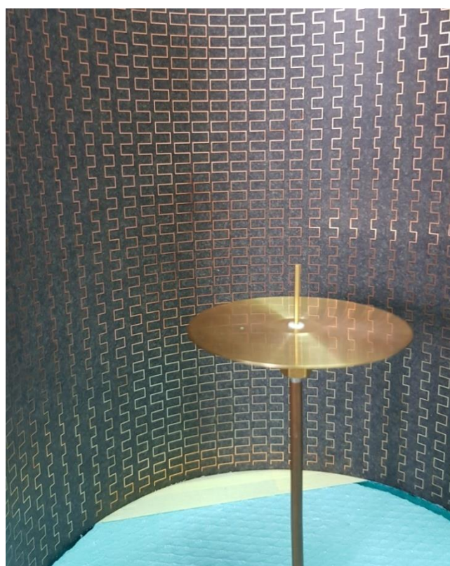
Fig. 6.16. Image of a cylindrical metasurface with a monopole feed antenna.
