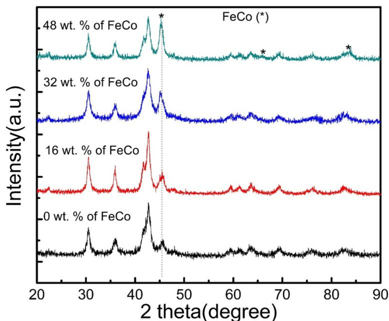
**Figure 1.** XRD pattern of FeCo coated SmCo<sub>5</sub> nanoflakes with different content of FeCo coating (wt % estimated from XRD analysis).
