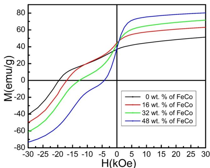
**Figure 4. Demagnetization curves of FeCo coated SmCo<sub>5</sub> nano-chips with different content of FeCo coating (wt % estimated from XRD analysis).**
