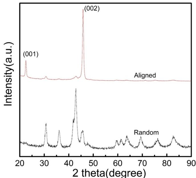
**Figure 6.** XRD patterns of randomly oriented  $\text{SmCo}_5/\text{FeCo}$  nanocomposite and aligned  $\text{SmCo}_5/\text{FeCo}$  nanocomposite chips in 2 Tesla magnetic field hardening in epoxy during alignment.
