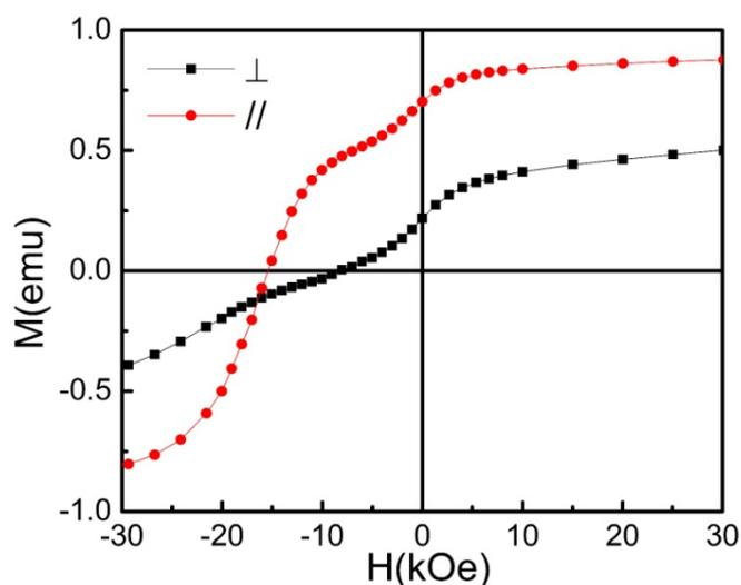
**Figure 7.** Demagnetization curves of  $\text{SmCo}_5/\text{FeCo}$  nanocomposite chips sample measured parallel and perpendicular to aligned field direction. The sample was aligned in magnetic field of 2 Tesla and was hardened in epoxy during alignment.
