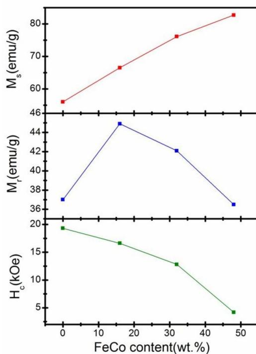
**Figure 5. Dependence of  $M_s$ ,  $M_r$  and  $H_c$  on content of FeCo on SmCo<sub>5</sub>/FeCo nanocomposite chips.**
