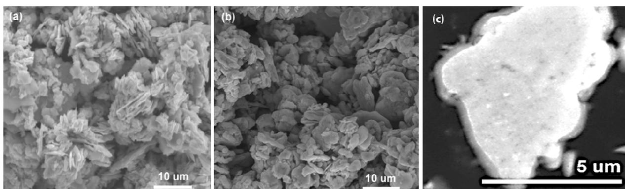
**Figure 2.** SEM images of (a) as prepared SmCo<sub>5</sub> nano-chips, (b) SmCo<sub>5</sub>/FeCo core/shell nano-chips and (c) a single SmCo<sub>5</sub>/FeCo core/shell chip.
