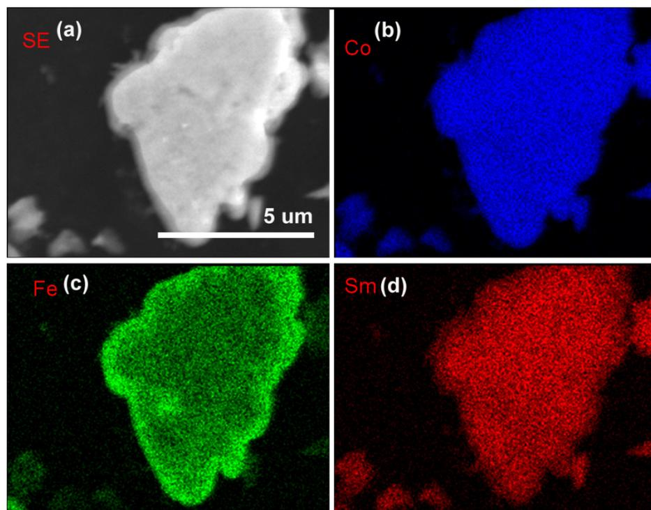
**Figure 3. (a) SEM image of a single  $\text{SmCo}_5/\text{FeCo}$  core/shell chip, and EDX element maps of the single  $\text{SmCo}_5/\text{FeCo}$  core/shell chip for (b) Co, (c) Fe and (d) Sm.**
