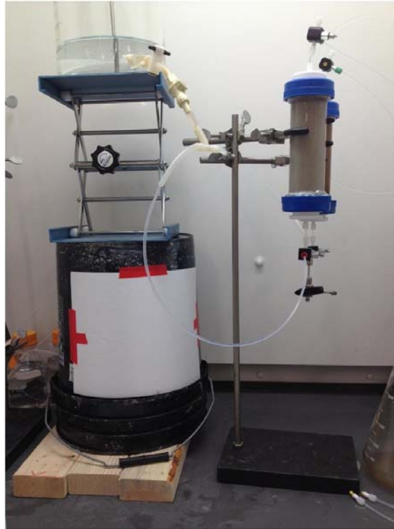
Figure 2.2.5. Head-driven column experiment setup with anoxic influent bottle above Federal Fine column #6 and Appling column #3 effluent line heights to establish gravity flow.
