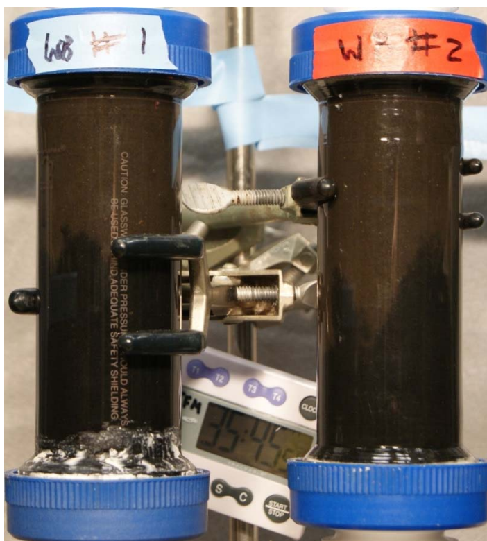
Figure 3.2.19. Head-driven columns packed with Webster soil after injecting 4 PVs of 800 mg/L iron (II) chloride and 73 PVs of reduced medium containing 100 mg/L S^{2-} (left, Webster soil column #1) or 44 PVs of reduced medium containing 100 mg/L S^{2-} (right, Webster soil column #2). The direction of water flow is upward, from bottom to top.
