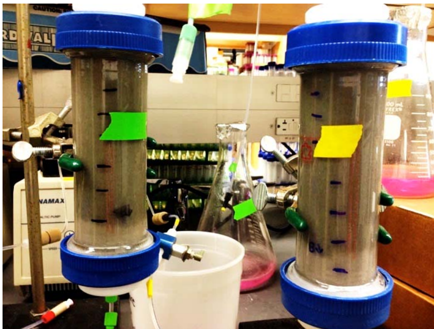
Figure 3.2.13. Difference in color between the inlet 2 cm (bottom) in Federal Fine Ottawa sand column #4 (right) and Federal Fine Ottawa sand column #5 (left) and the remainder of the column (above) indicating FeS precipitate. The direction of water flow was upward, from bottom to top.
