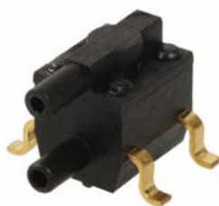
Figure 2.2.3. Image of a differential pressure sensor that was attached to the column influent and effluent to monitor changes in pressure and in turn, permeability due to FeS precipitation and subsequent oxidation, when applicable.
