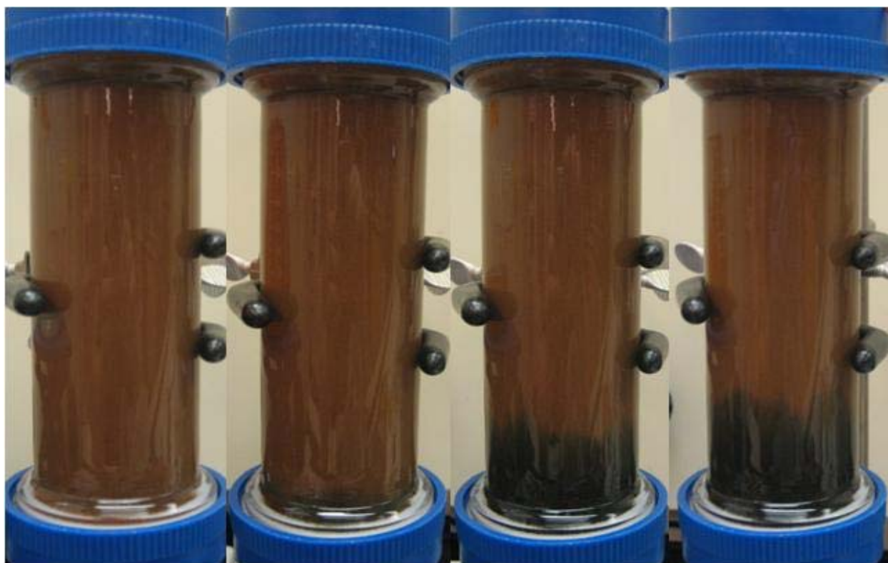
Figure 3.2.3. Appling soil column (15 cm) after reduced medium (11 PV of 3 mg/L sulfide, then 22 PV of 140 mg/L sulfide) was injected (flow direction from bottom to top), with black precipitate (FeS) evident in the first 5 cm of the column. Pictured from left to right: 0 PV, 15 PVs, 26 PVs, 33 PVs.
