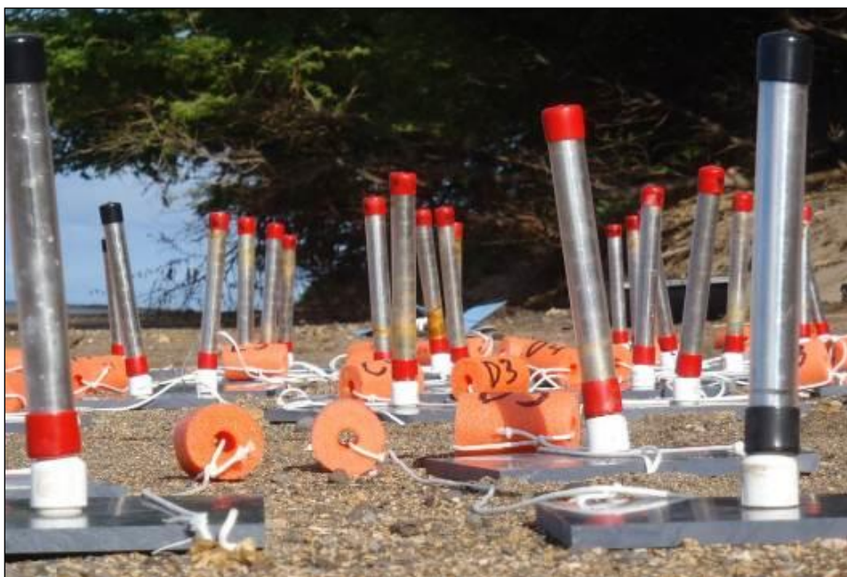
Figure 30. The magnet and sheath assemblies attached to baseplates with identifying location floats prior to deployment.
