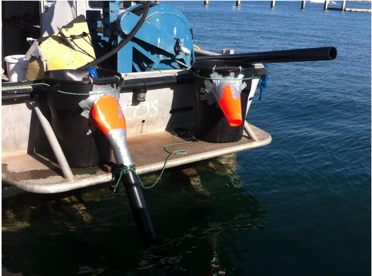
Figure 11. Continuous flow stations developed for the tracer material deployment on the swim platform of the Ecos.
