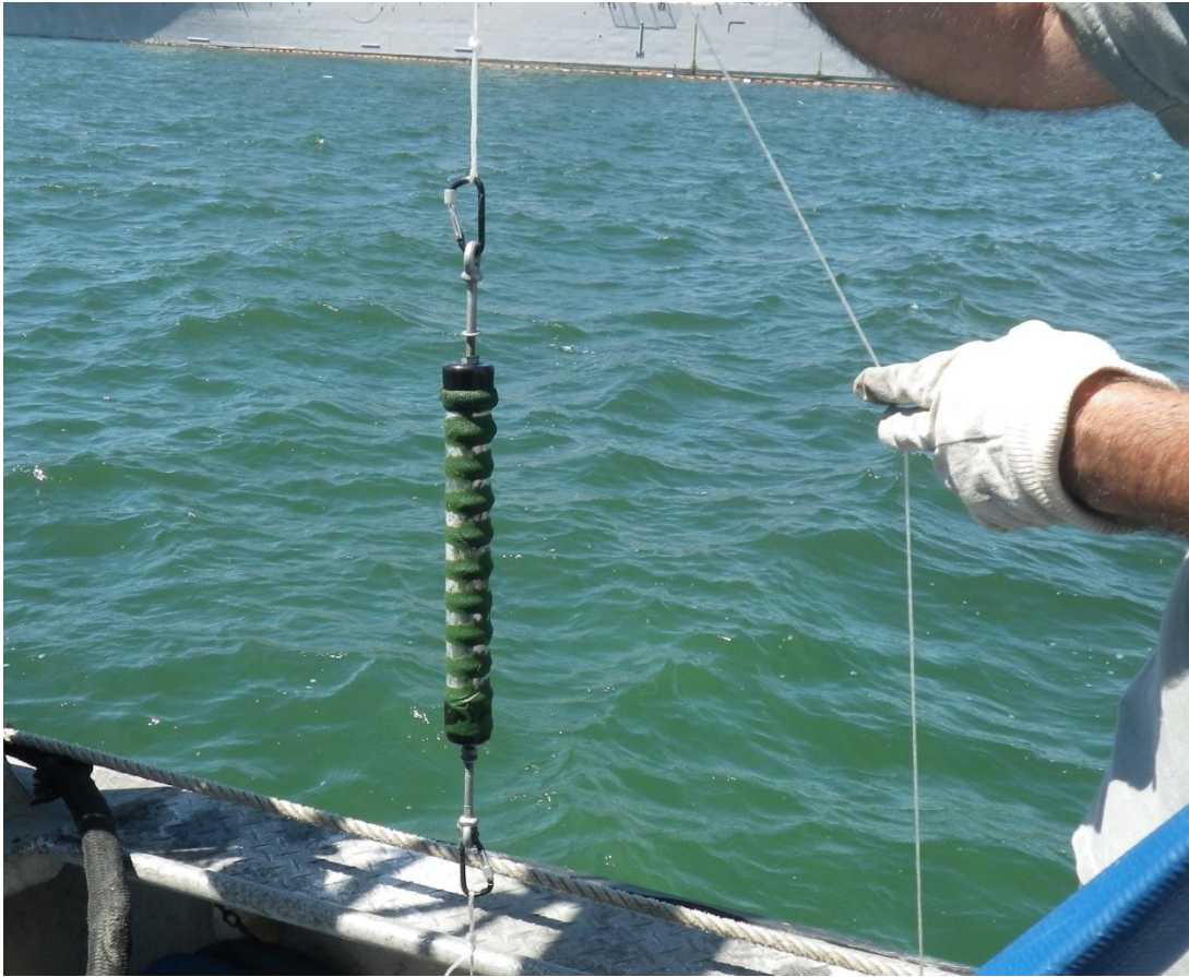
Figure 13. Recovered magnet showing tracer material that has been collected while submerged.
