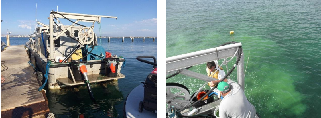
Figure 20. (Left) Setup for tracer release done from stern swim platform from 32 gallon mixing container with overflow through 4 inch PVC pipe so tracer released just below the water surface. (Right) High flow pump with 2 inch fire hose (blue hose) mixes and disaggregates tracer to deliver tracer plume to surface waters 10-50 meters from outfall 20 (visible buoy at site T3-2).
