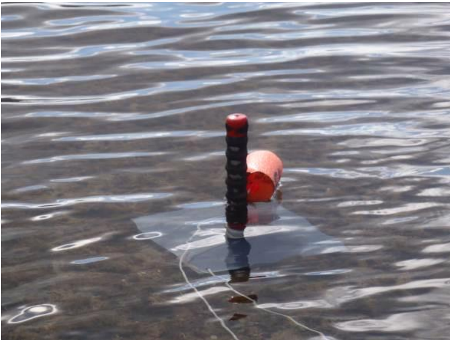
Figure 8. A vertical bed-frame mounted magnet to capture tracer moving in the bottom boundary layer at the second demonstration site.
