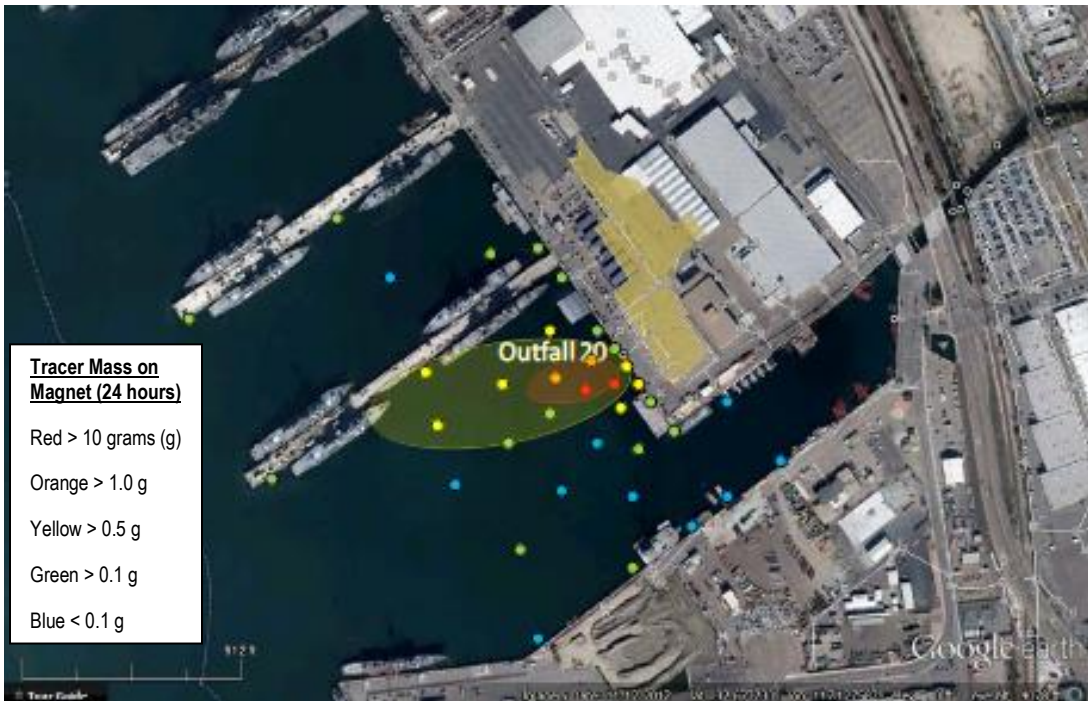
Figure 24. Colored post map of magnet results 24 hours after tracer release near Outfall 20.
