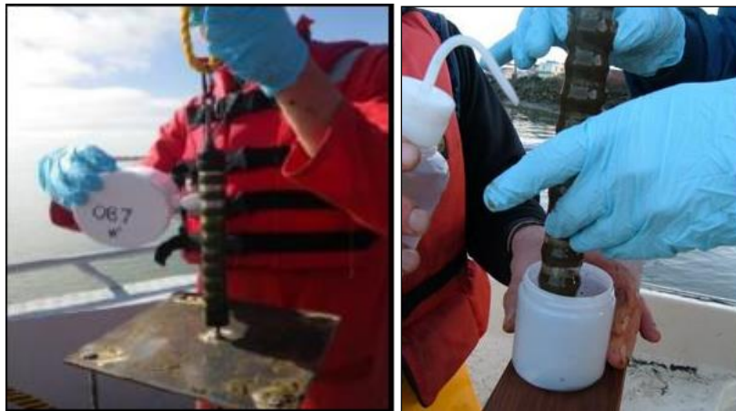
Figure 32. Tracer collection from magnets.
