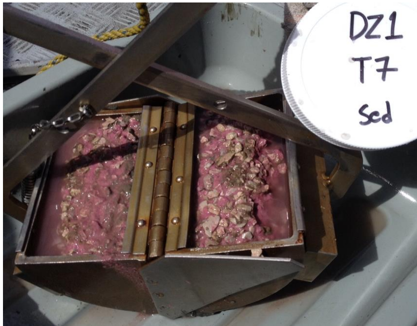
Figure 33. A sediment grab from the middle of AquaGate deployment zone (DZ1) 6 days following placement showing the pink tracer has been released from the white pea gravel at the sediment surface.
