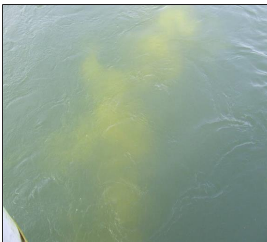
Figure 6. Sampling suspended tracer can be done directly using a pole magnet dipped into this cloud of green tracer.
