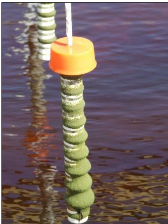
Figure 5. In situ capture of tracer using a submersible magnet.
