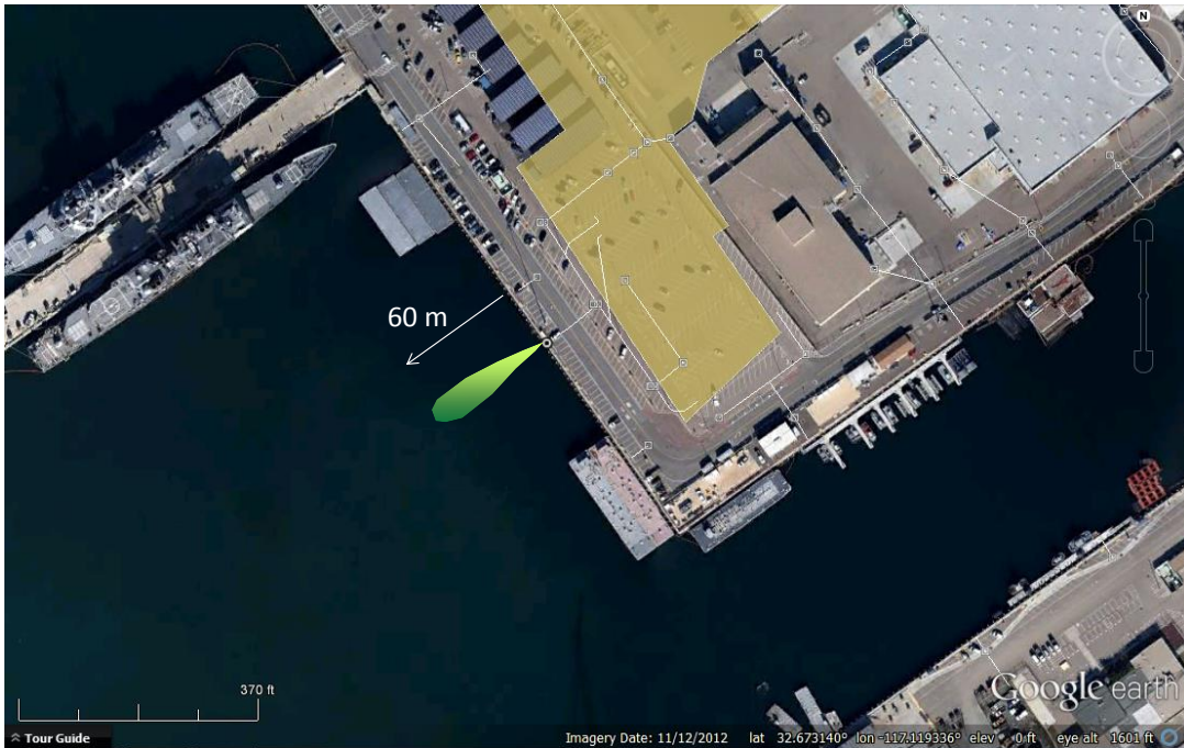
Figure 18. Proposed Outfall 20 location, with drainage basin (top, in yellow), and associated discharge zone plume depicted in the Paleta Creek area south of Pier 8 (bottom, in green).
