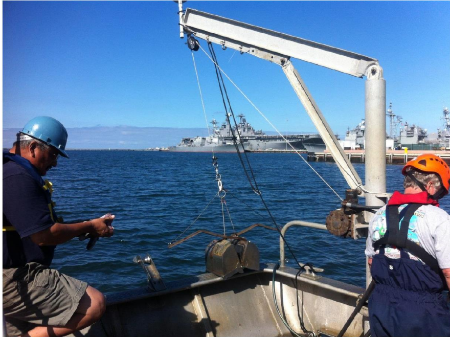
Figure 7. Use of sediment grab to monitor deposition of tracer at the first demonstration site.
