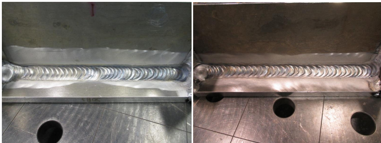
Figure 9. Example 6055-5083 restrained-tee welds using C138H (left) and C139H (right)
