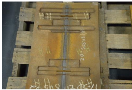
Figure 6. Phase 1-Plate Marked Samples for Standardized Weld Characterization Tests.
