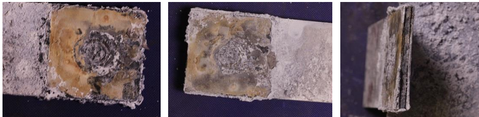
Figure 9. UPJ8-2 (bare Mg to bare Al6013) after eight-weeks of accelerated corrosion exposure.
