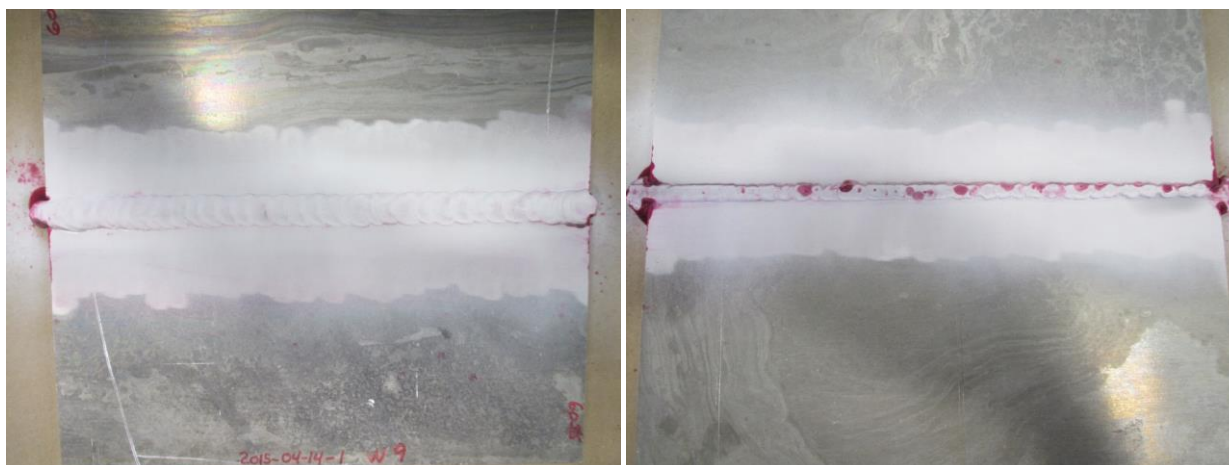
Figure 4. Example face (left) and root side (right) penetrant inspection for 6055-T6 GTA welded with C138H
