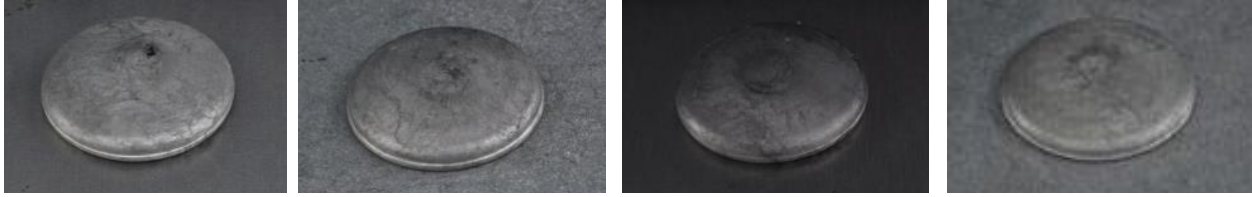
Figure 18. UCR head formations for four unique material/coating configurations.
