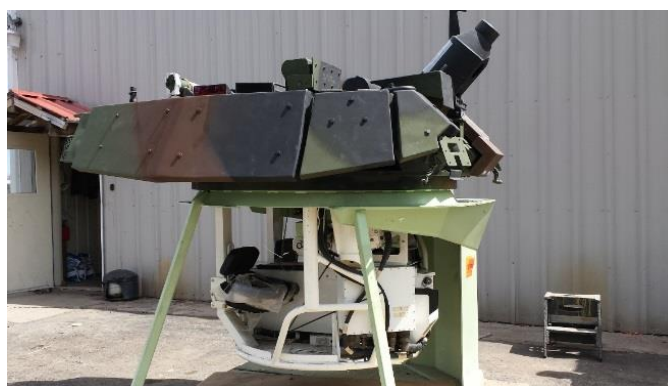
Figure 5. Assembled Lightweight Turret with Basket and Armor in a Turret Stand.
