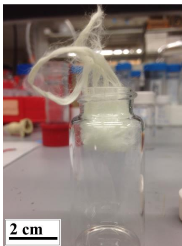
Figure 5. Image Showing the Yarn-like Nature of the Flex – sulfur Wires (Flex-SWs).
