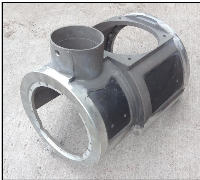
Figure 13. Gunner Rotor assembly casting and welding.
