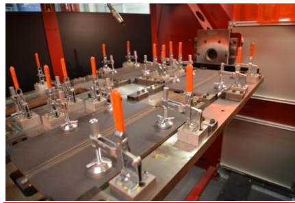
Figure 1. Fixture for Robotic Welding of Phase 1 plate.
