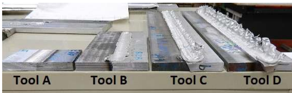
Figure 4: Side view of FSW's made with Tools A, B, C and D
