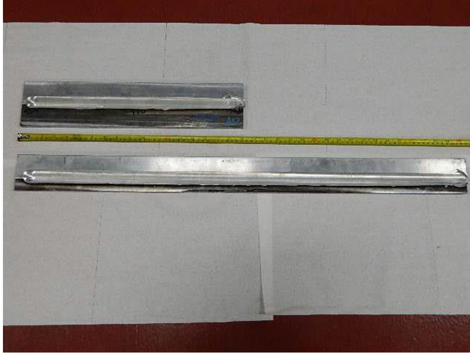
Figure 6: Sample of 18'' and 36'' long bimetallic FSW's
