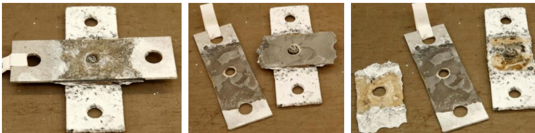
Figure 10. UPJ8-2 (bare Mg to bare Al6013) after twelve-weeks of accelerated corrosion exposure.
