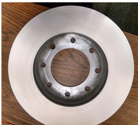
Figure 13. FeMn4 Brake Rotor Coating on GDOT Rotor.
