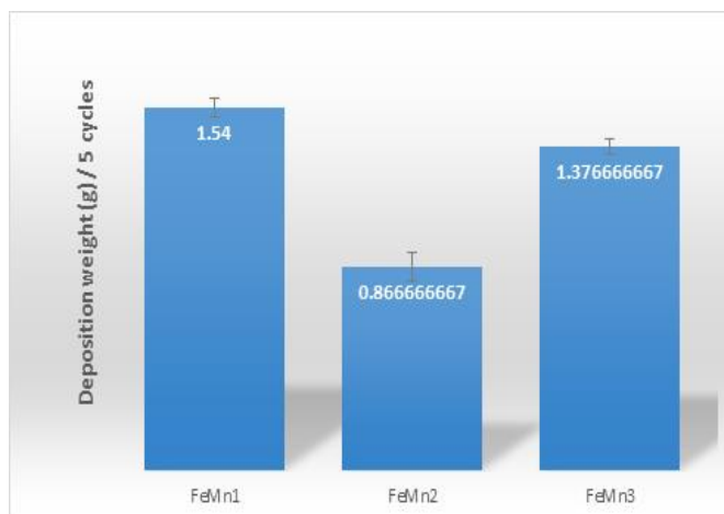
Figure 5. Deposition Weights for Various FeMn Alloys.
