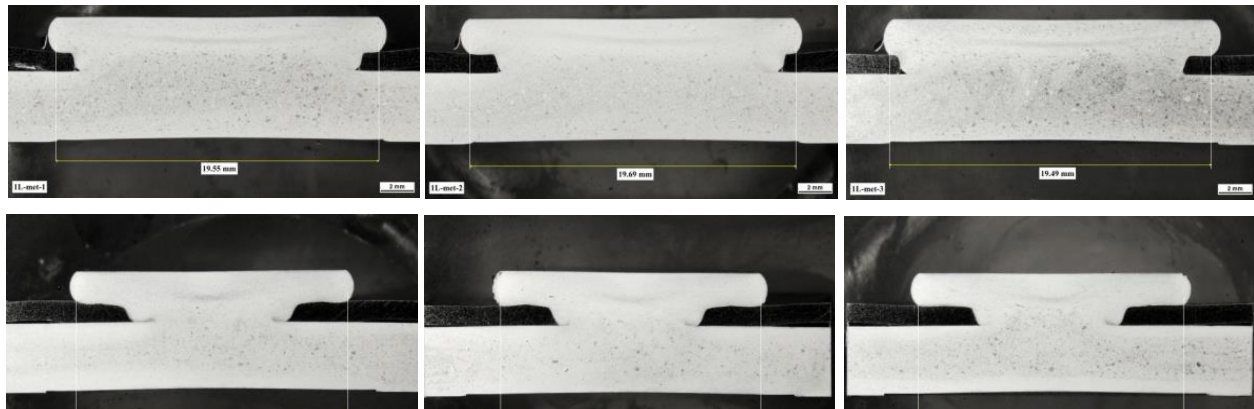
Figure 16. Metallurgical cross-sections of oval boss UPJ joints through the transverse axis (top) and the longitudinal axis (bottom).
