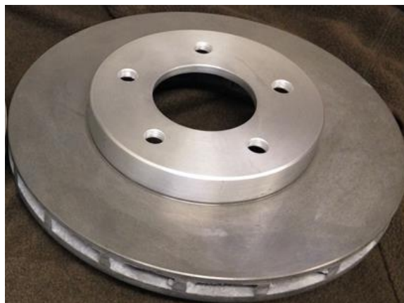
Figure 7. Prototype Internally Vented MMC Rotor.
