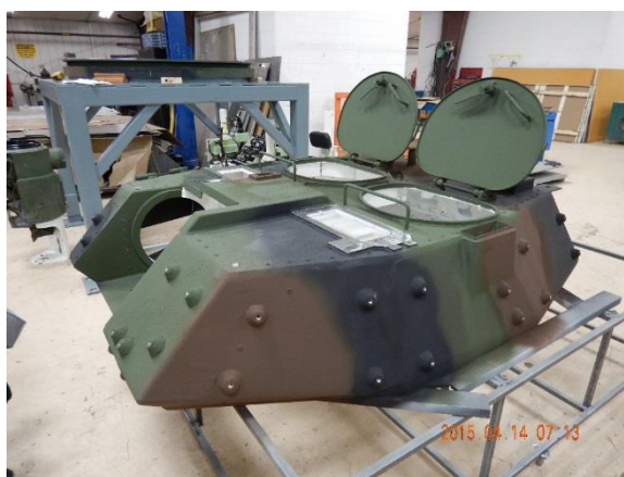
Figure 4. Assembled Lightweight Turret Structure.
