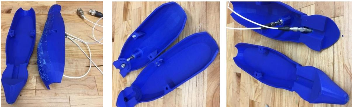
*Figure 19. Interior overview of the RTD prototype showing sensor mounting and wiring*
