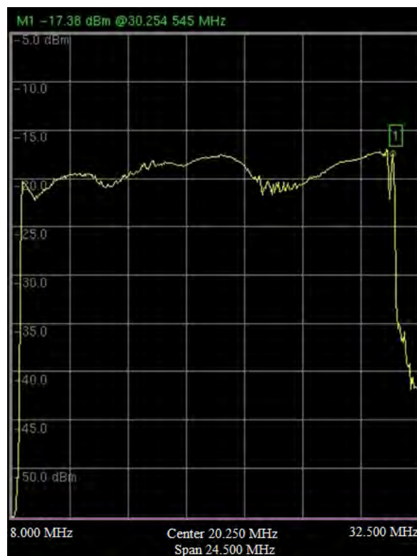
Figure 4-57 Measurements of generated signal power of prototyped N-type non-Foster antenna-transmitter with antenna-emulating network operating within 9 to 30 MHz bandwidth
