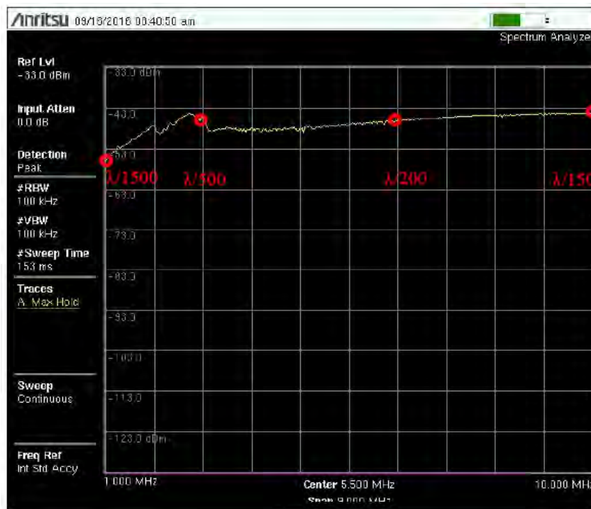
Figure 4-61 Measured normalized radiated power of prototyped N-type non-Foster antenna-transmitter with a short monopole antenna on a conducting plane at 1 to 10 MHz bandwidth
