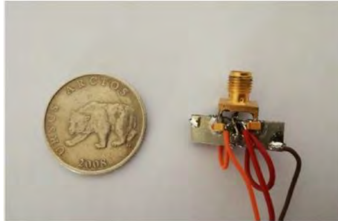
Figure 3-19 A photo of an RF demonstrator of stable negative band-pass capacitor
