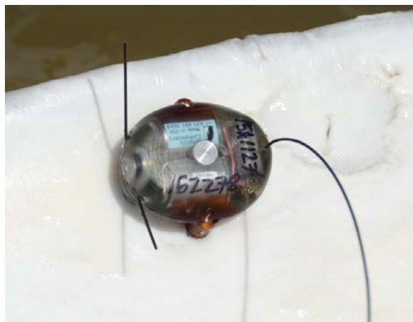
Fig. 5. Fastloc GPS LIMPET design model 333B with symmetrical V GPS dipole whip antenna configuration.
