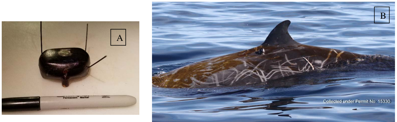
Figure 7. A) Fastloc GPS-LIMPET tag in the SPLASH10-F-333B configuration. B) GPS-LIMPET deployed on an adult male Cuvier's beaked whale (ZcTag053).
