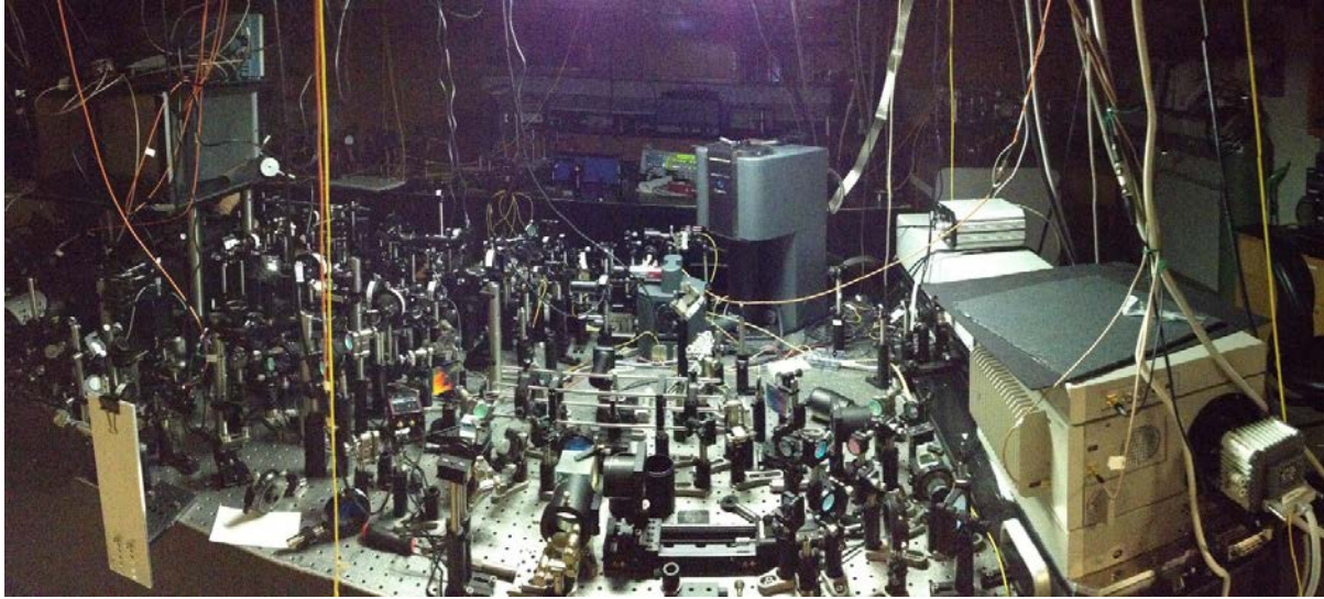
Fig. 6. A picture of the optical spectroscopy system integrated with the Montana Ins. cryostat and ultrafast excitation laser. It includes in both the excitation path and collection path control of the laser or signal beams' power, spectral width and polarization. The signal is collected by confocal-spectroscopy then sent for real-space or Fourier-space imaging selected by a flip mirror, for spectrally resolved and/or time-resolved measurements, first and second-order interference spectroscopies.
