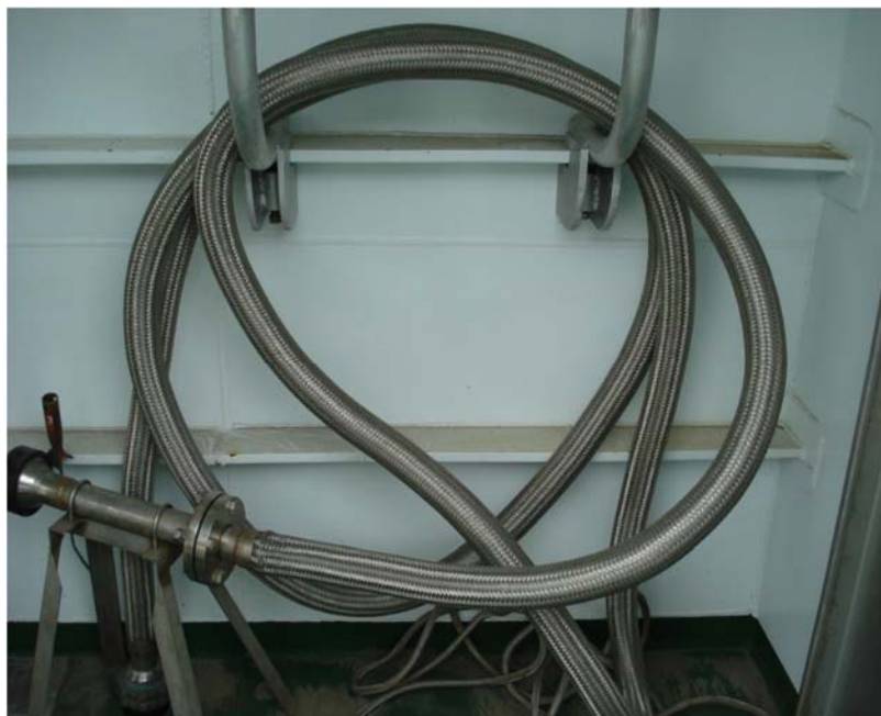
Figure C-4. On deck stowage of LNG bunkering hoses.
