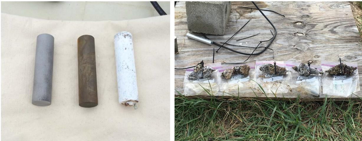
Figure 18 – 1-in steel surrogate with various corrosion (left), and biofouling (right) examples
