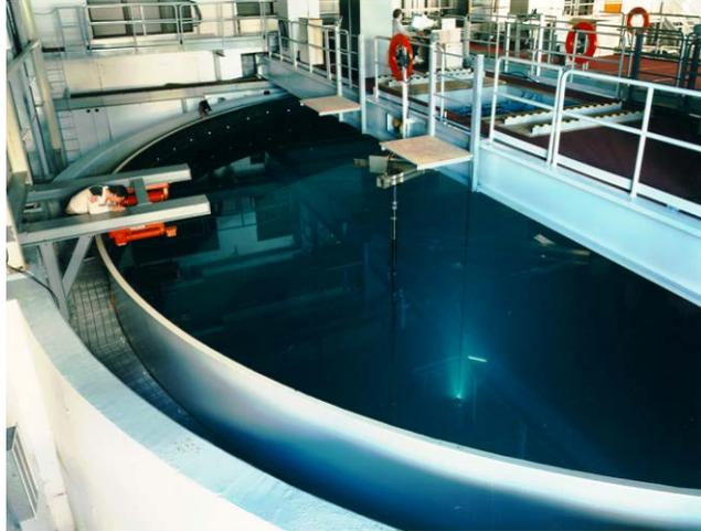
Figure 25 – NRL Laboratory for Structural Acoustics. A one-million gallon pool facility with adiabatic walls and acoustic coatings, vibration isolation system, and complex acoustic scanners, sources, and processing algorithms.
