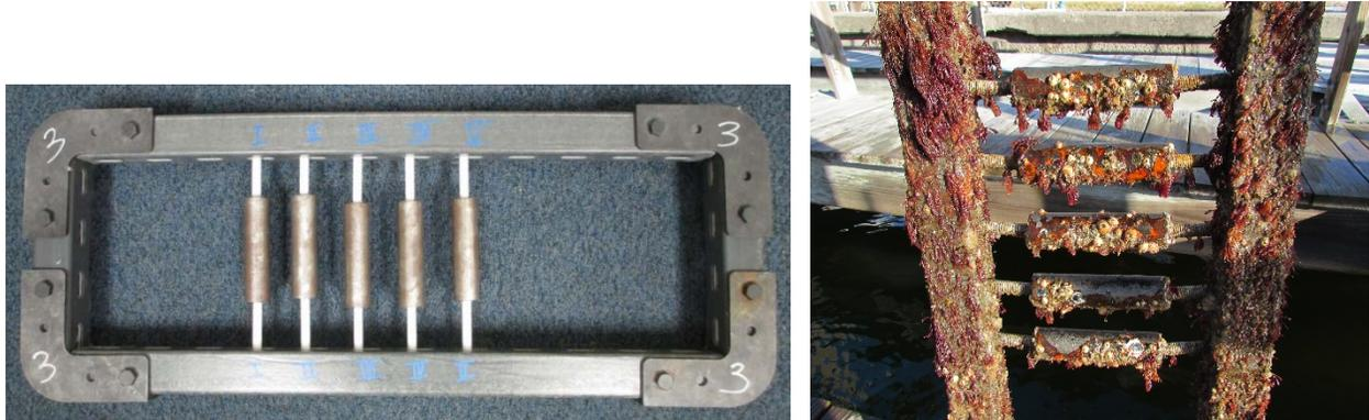
Figure 6 – (left) a rack of UXO surrogates prior to exposure, (right) a rack of UXO surrogates after 8 weeks of exposure.
