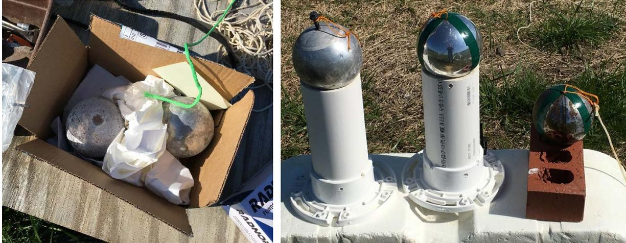
Figure 22 – Calcareous Films Grown on 4-inch Diameter Spheres (left) Steel and Aluminum (left to right), and (right) Aluminum with Calcareous film, bare Aluminum, and bare Steel (left to right).
