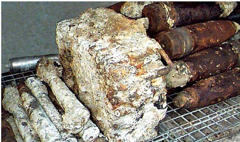
Figure 1 – Examples of fouled and corroded munitions recovered from underwater.
