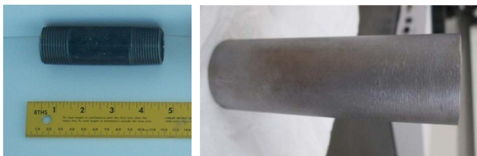
Figure 3 – (left) Small ISO, (right) solid steel surrogate.
