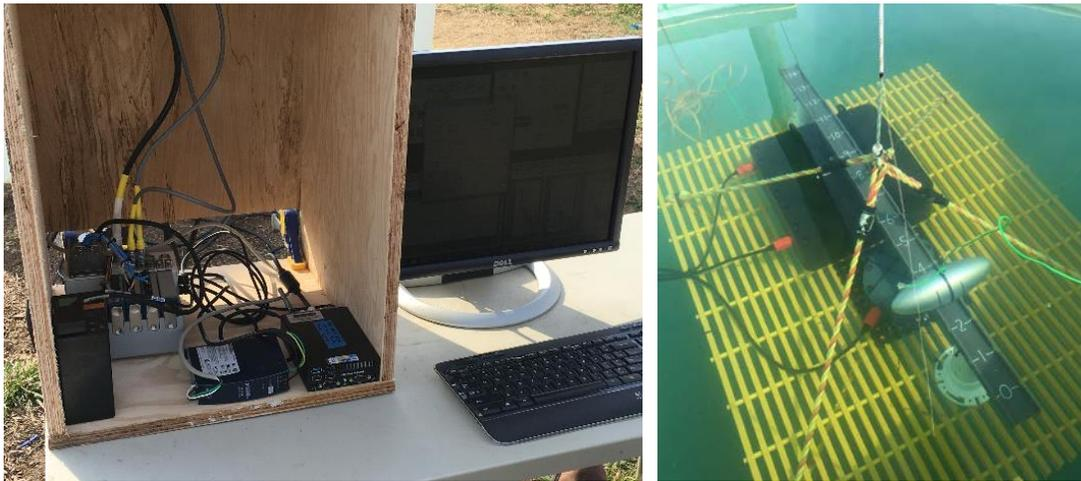
Figure 11 – (left) MR-2409 DAQ and electronics, (right) MR-2409 sensor assemblies in the water with an ellipsoidal test object in position.
