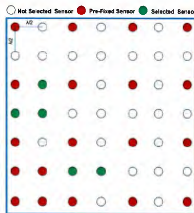
Figure 9: 24 element worst performing hybrid antenna array (19 prefixed, 5 selected)
