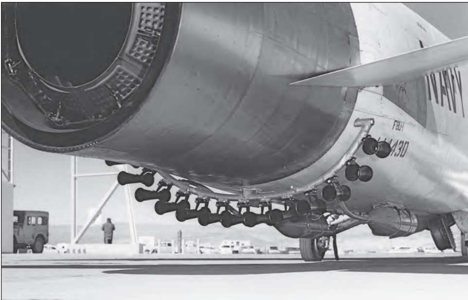
Project DIRTY aluminum-powder dispenser on an F8U-1 aircraft.
