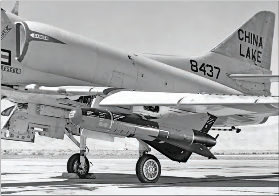
Walleye AGM-62 glide weapon on A-4 Skyhawk aircraft.
