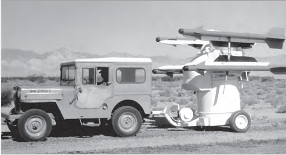
Jeep in SNORT area towing Ospreys with 5-inch motors on Mk-45 tracking-camera mount, 4 June 1962.
