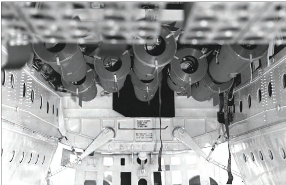
Cyclops II dispensers in bomb bay of A-3B aircraft.
