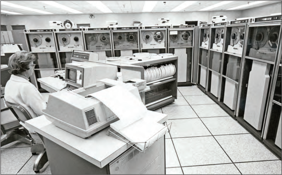
A few of the tape decks for NOTS' mainframe computer in the 1960s.
