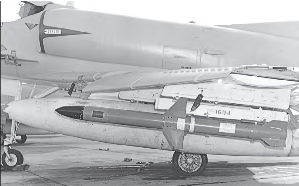
Shrike Missile AGM-45A on VX-5 A-4E aircraft, Armitage Field, China Lake, 1965.
