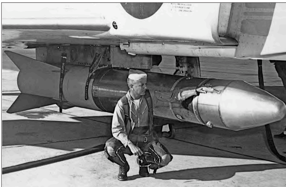
Lieutenant Al Newman with HIHOE on a Caleb vehicle mounted on a YF4H-1 Phantom, Naval Air Facility, China Lake, July 1962.
