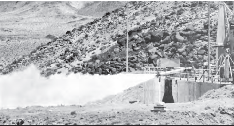
Skytop static firing test of large composite-propellant motor.
