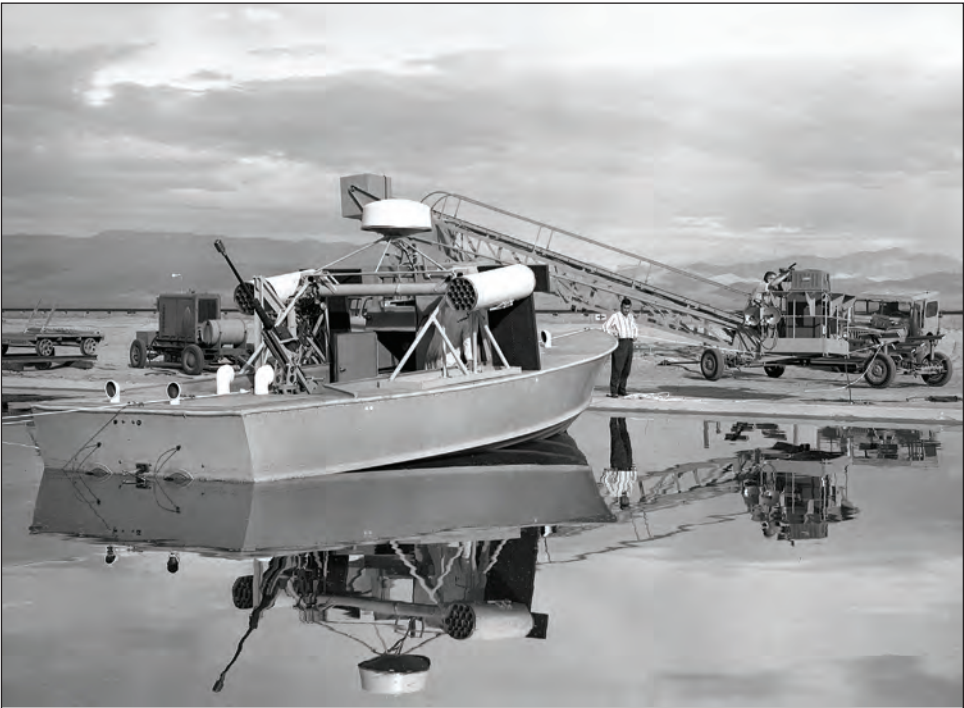
SWAB carrying original 2.75-inch rocket canisters, with Raymond Laidler (standing by the boat) and John Boyle (looking through a scope at right), at SNORT Reservoir.
