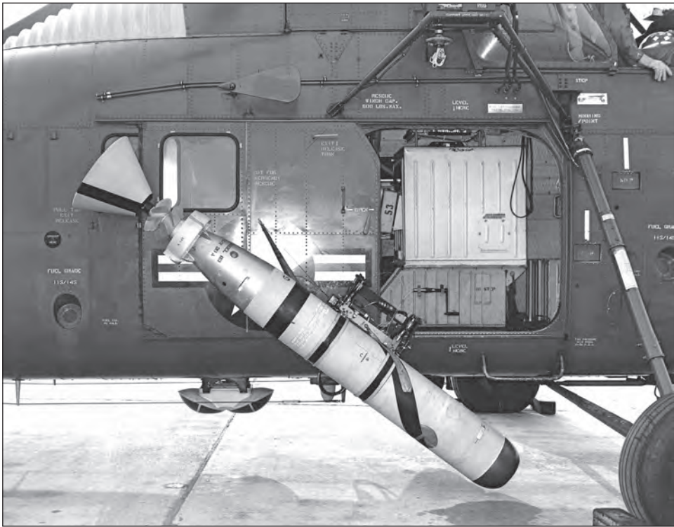
Torpedo Mk 46 rigged for an instrumented air drop from a UH-34 helicopter.
