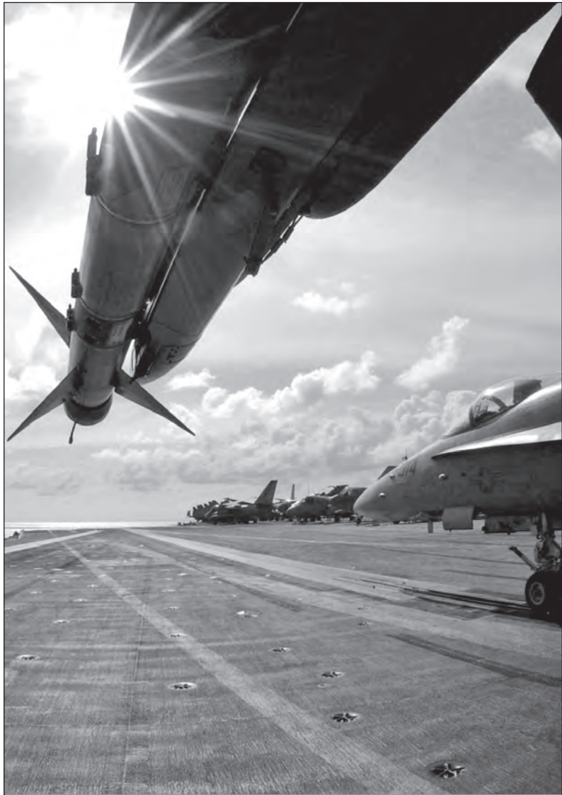
Sidewinder AIM-9M on an F/A- 18C Hornet aircraft, flight deck of USS Kitty Hawk (CV 63), 17 February 2003.
