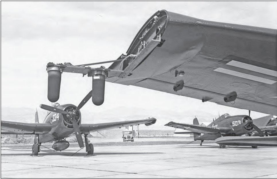
F6F-5K drone rigged with thermic pots, 2 May 1957.
