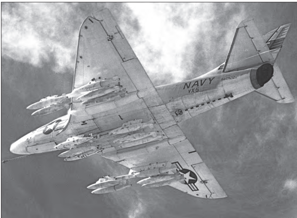
VX-5 A-4 aircraft with Multiple Carriage Bomb Racks loaded.
