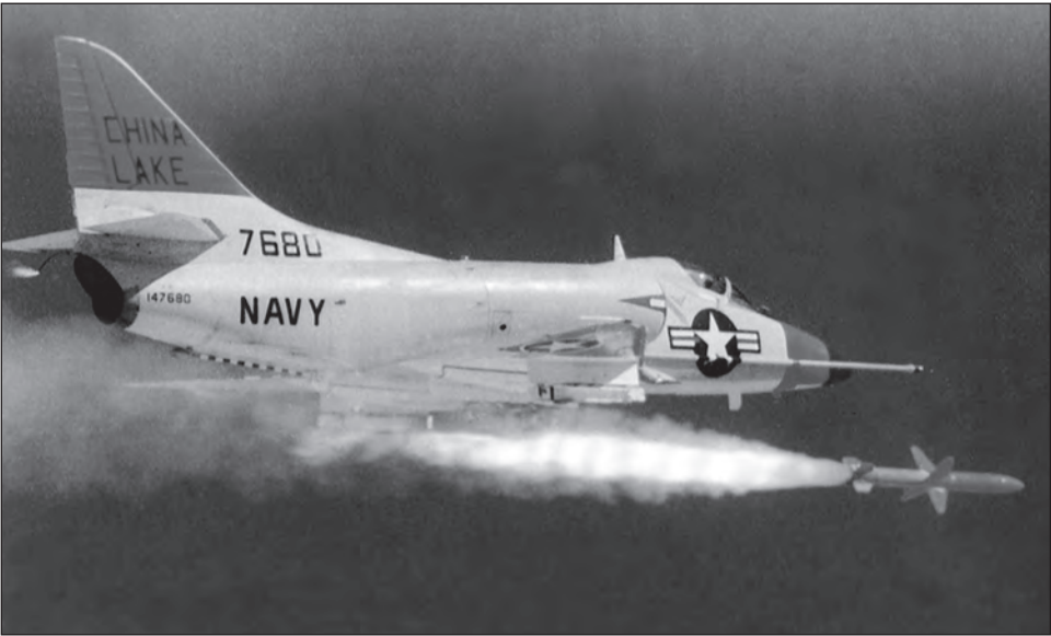
Project Pilot Tony Tambini firing Shrike from an A-4C aircraft in a test at China Lake, 12 June 1964.
