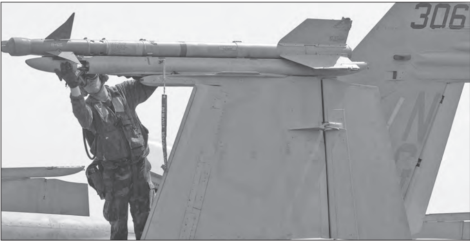
Aviation ordnanceman checking Sidewinder missile mounted on F/A-18C aircraft, Strike Fighter Squadron 146 aboard USS John C. Stennis (CVN-74) in the Persian Gulf, May 2007—more than half a century after the NOTS-developed missile's first successes.
