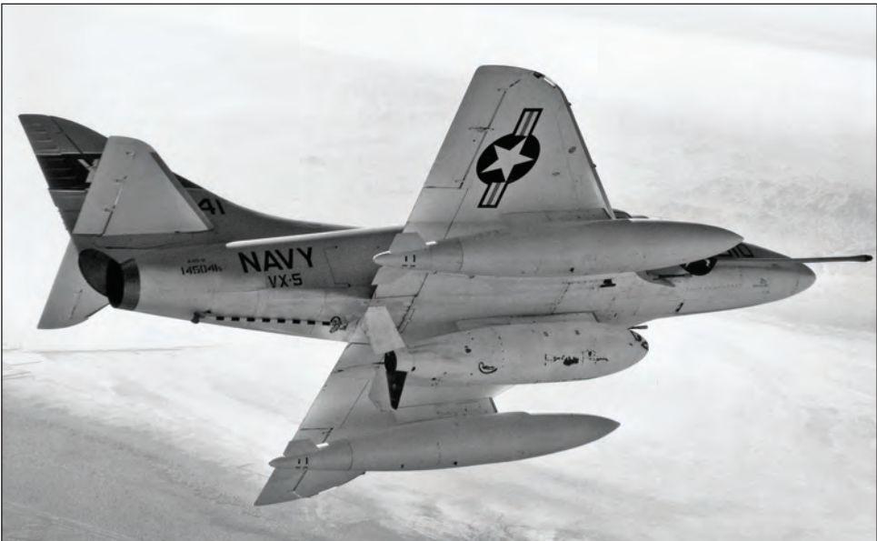
VX-5 A4D-2 Skyhawk in flight with a Mk-7 nuclear shape (T-63) on the centerline, circa 1959.
