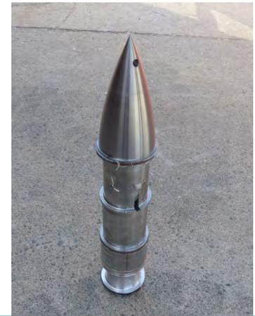
Projectile recovery after the test
