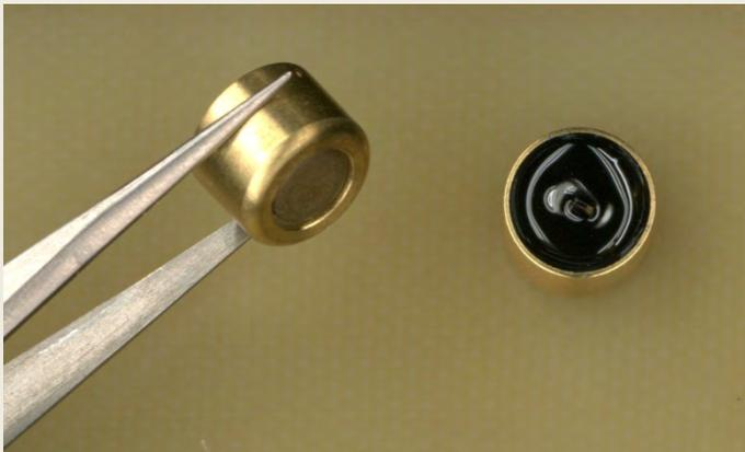
Finish and tested laser diode primer
