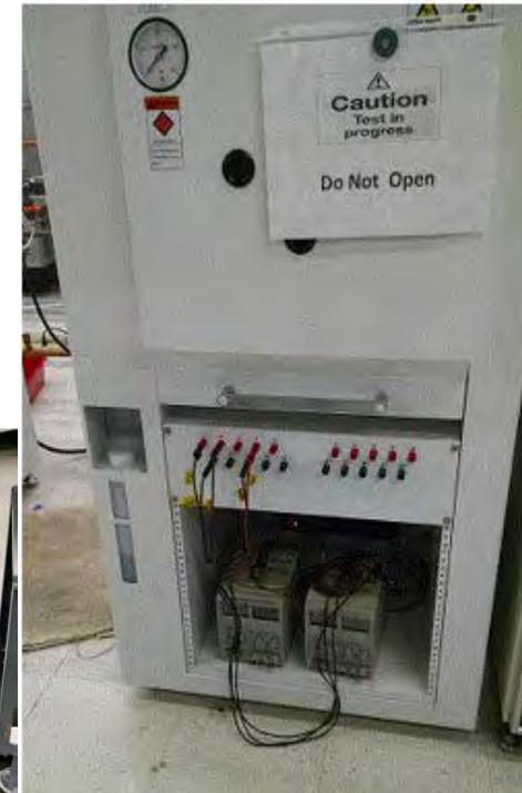
**HAST Chamber with humidity control and voltage bias interface. Tested at HASTest Inc.**
