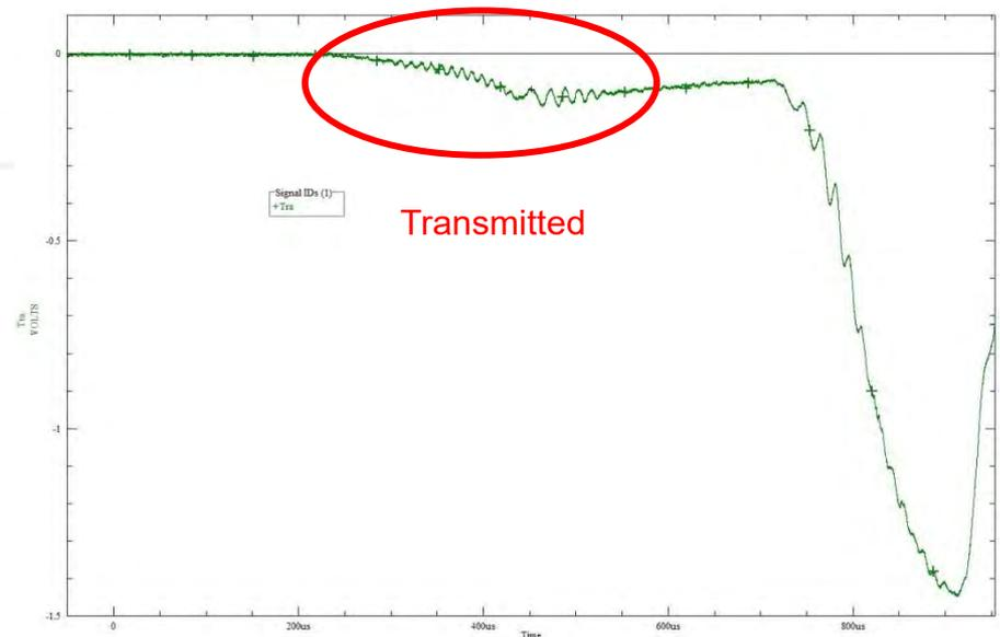
Raw waveforms for incident, reflected and transmitted are isolated and used in calculation of Frequency Response Function (FRF), analysis scheme suggested by Vesta Bateman (Sandia TR 1437).
