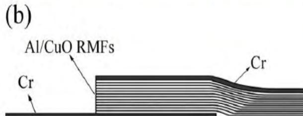
the igniter. The ignition delay time and total released energy of the igniter discharged in 40 V are 0.7 ms and 482.34 mJ, respectively. For one igniter, the energy released by chemical reactions is accounted for 21% of the total energy, which can be improved by adjusting the deposition conditions of Al/CuO RMFs and by tuning the Al deposition to reach a stoichiometric reaction. Furthermore, the explosion temperature could keep an approximately constant value of 3500 °C for 1.4 ms.
