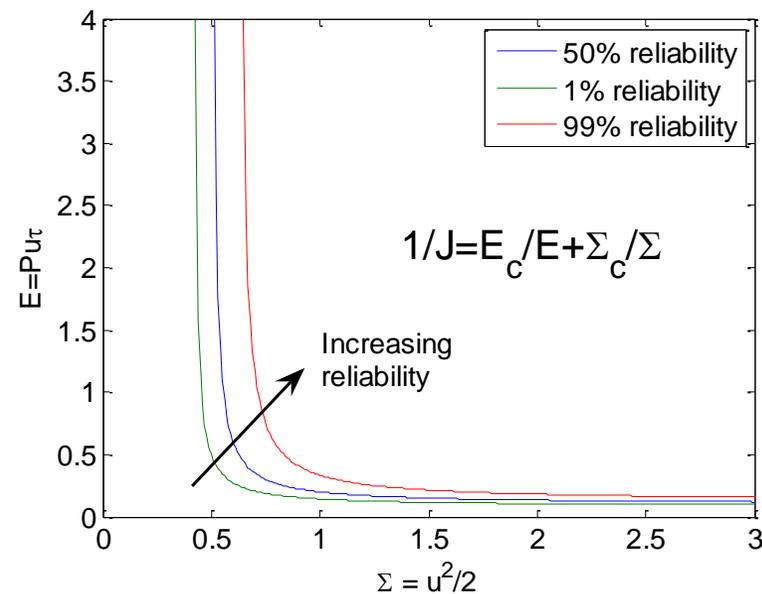
$E_c$  (critical minimum energy) &  $\Sigma_c$  (critical minimum 'power') are defined by the acceptor explosive material.  $E$  &  $\Sigma$  can be calculated from variable flyer and gap tests and inherent explosive properties.
