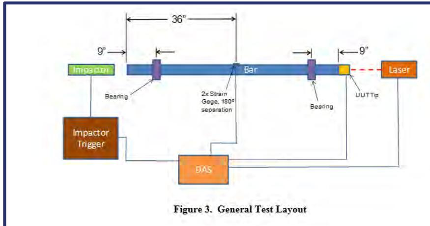
Figure 3. General Test Layout
