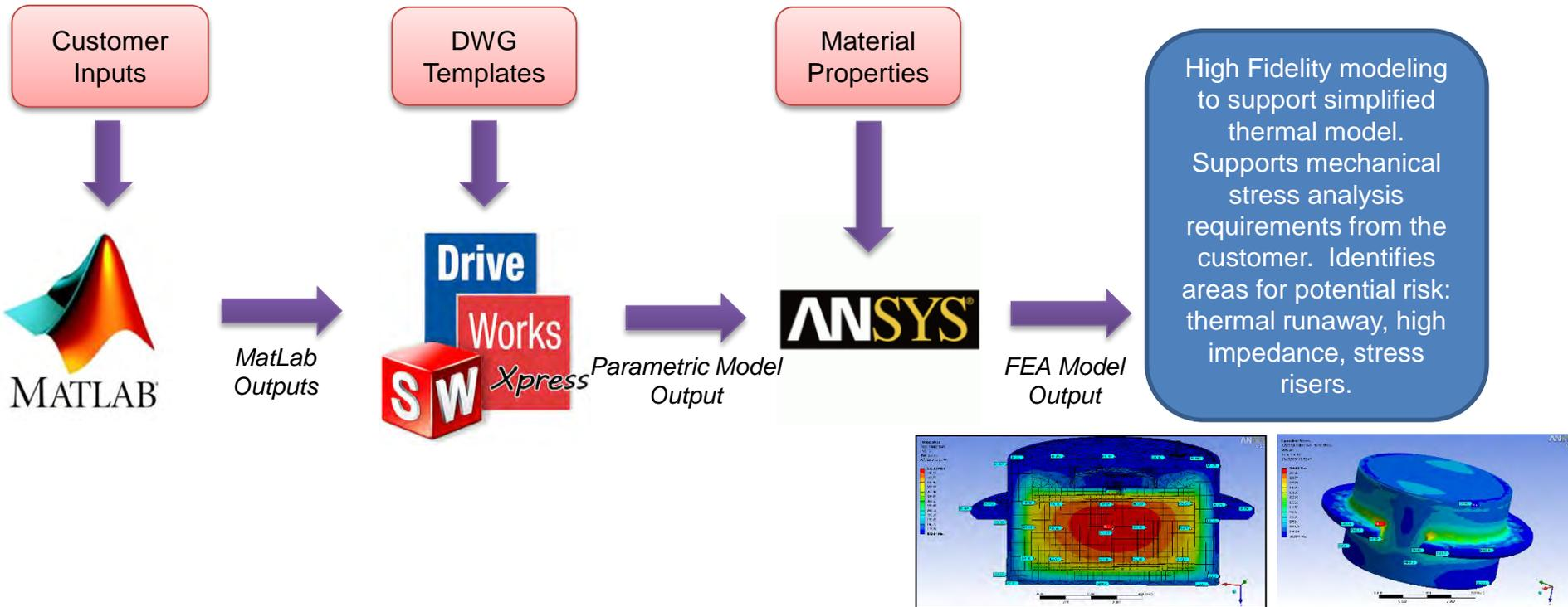
*Using a combination of the latest software packages, EAS can generate thermal and mechanical models to reduce cost and time to PDR.*
