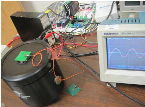
\* **Test setup with vibrator and frequency monitor**
