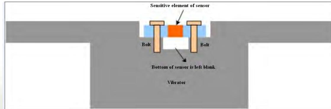
Fig.3 Schematic of the installation of the sensor
