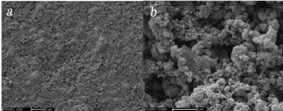
Cu film by magnetron sputtering
