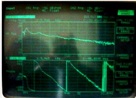
Broadband signal from shaker is transmitted into the sample. Signal input vs. output is recorded for amplitude and phase shift for **10Hz-25Khz**
