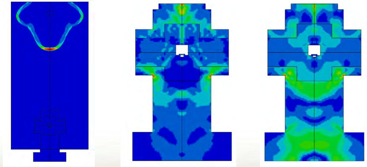
Fig.6 Stress wave propagation in the structure
