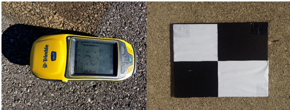
Figure 17: Trimble geo 7x (left) and manual Ground Control Point (30 x 25 cm).
