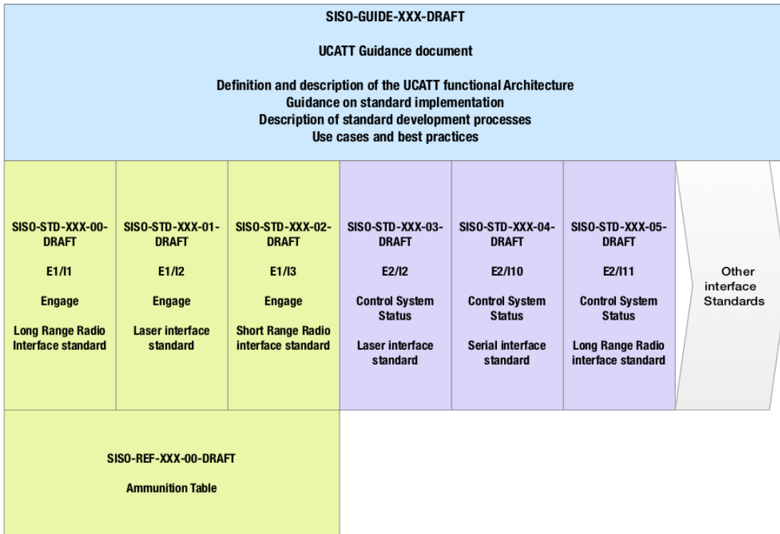
Figure 1. Diagram showing the projected UCATT family of standard, guidance and reference products
