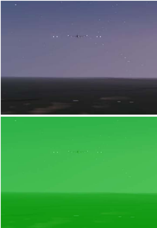
Figure 1: Simulated images of aircraft in low ambient lighting conditions without (top) and with (bottom) monochrome green backlight LCD bleed-through. Note the decreased visibility of low contrast scene content.
