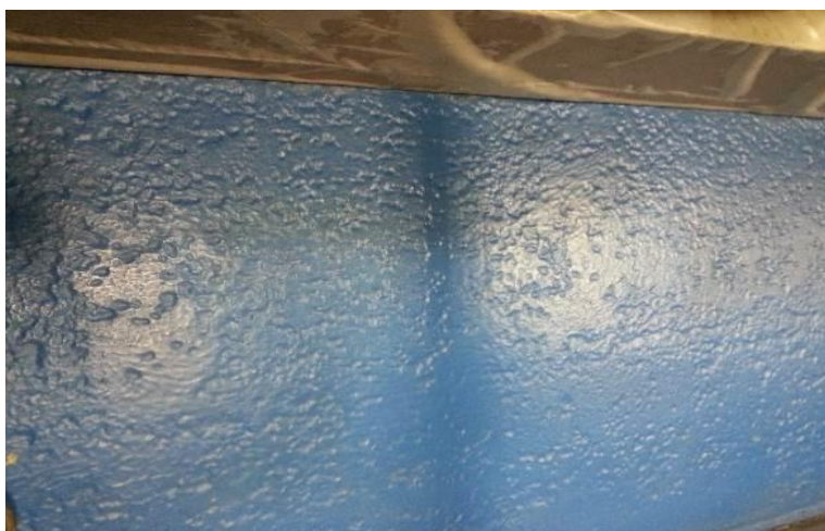
Figure 30: The STF bed is made of rough (pitted), painted steel.
