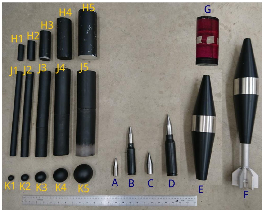
Figure 4: The surrogates (blue) and canonical-shape (yellow) objects tested in the initiation of motion experiments.
