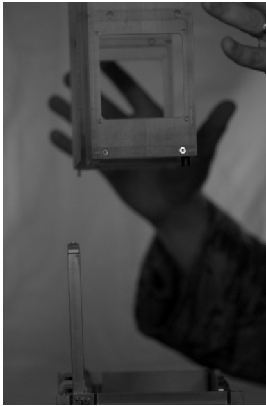
Figure 91. Vertical Ejection of 3-D Printed 6U Chassis
