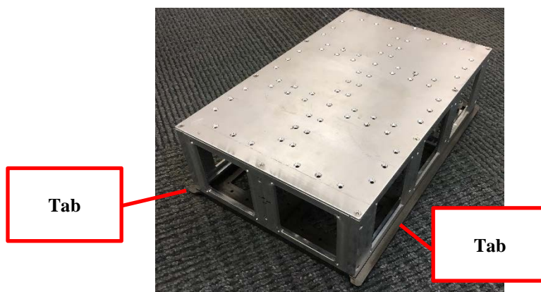
Figure 8. 6U CSD-Compatible CubeSat Chassis with Tabs [12]
