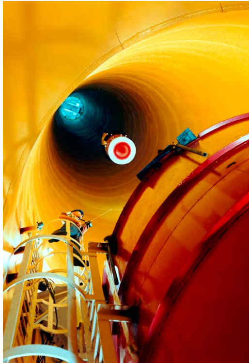
Figure 28. NASA GRC 5.18 s Drop Tower with Experiment Being Hoisted [32]
