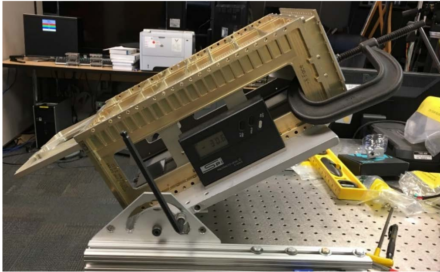
Figure 73. CSD Attached to Tilting Apparatus with Inclinometer
