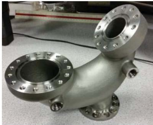
Figure 3: Additively Manufactured Fuel Mixer [16]
