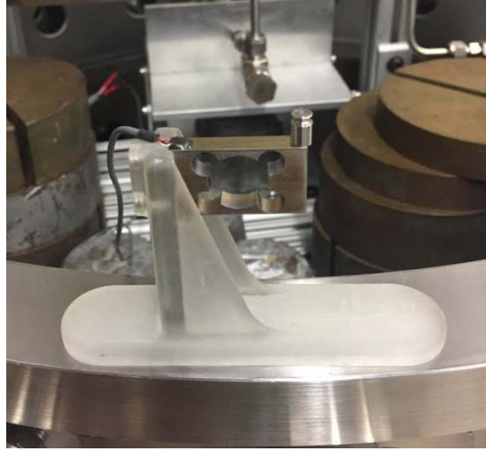
Figure 19: Load Cell Mounted for Calibration
