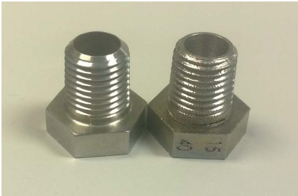
Figure 4: Machined Nozzle (Left) and DMLS Nozzle (Right)
