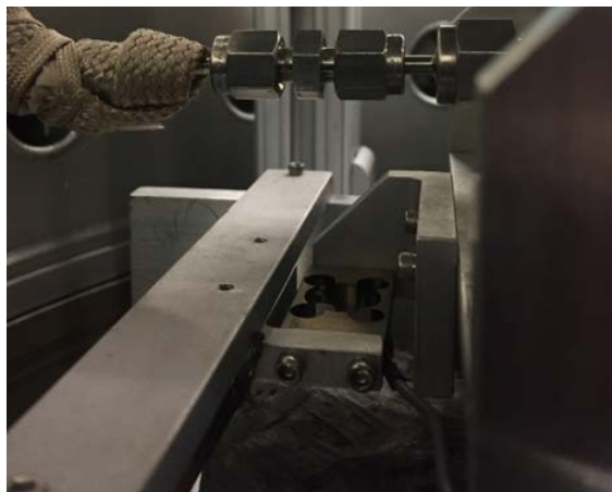
Figure 16: Load Cell Mounted in Thrust Stand
