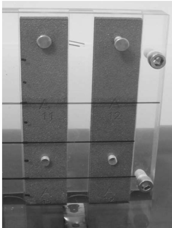
Figure 14. Experimental Setup for simple wicking ability test for additively manufactured “porous bars”.
