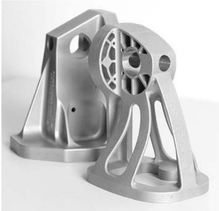
Figure 6. Comparison of traditionally manufactured (rear) and AM (front) parts and size and weight savings possibilities. [14]
