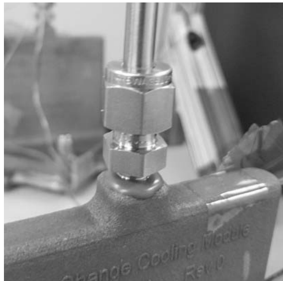
Figure 23. Method used to ensure heat pipe held pressure without leaking.
