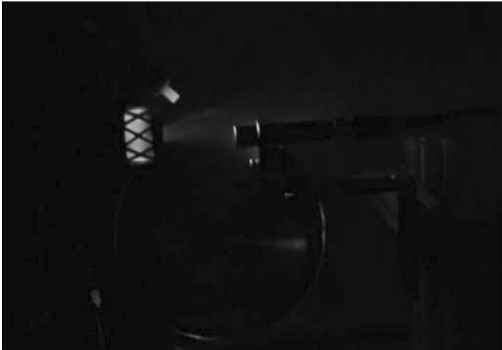
Figure 41. A BIT-1 Ion Thruster During Operation at Busek from Muilenburg [6:92]
