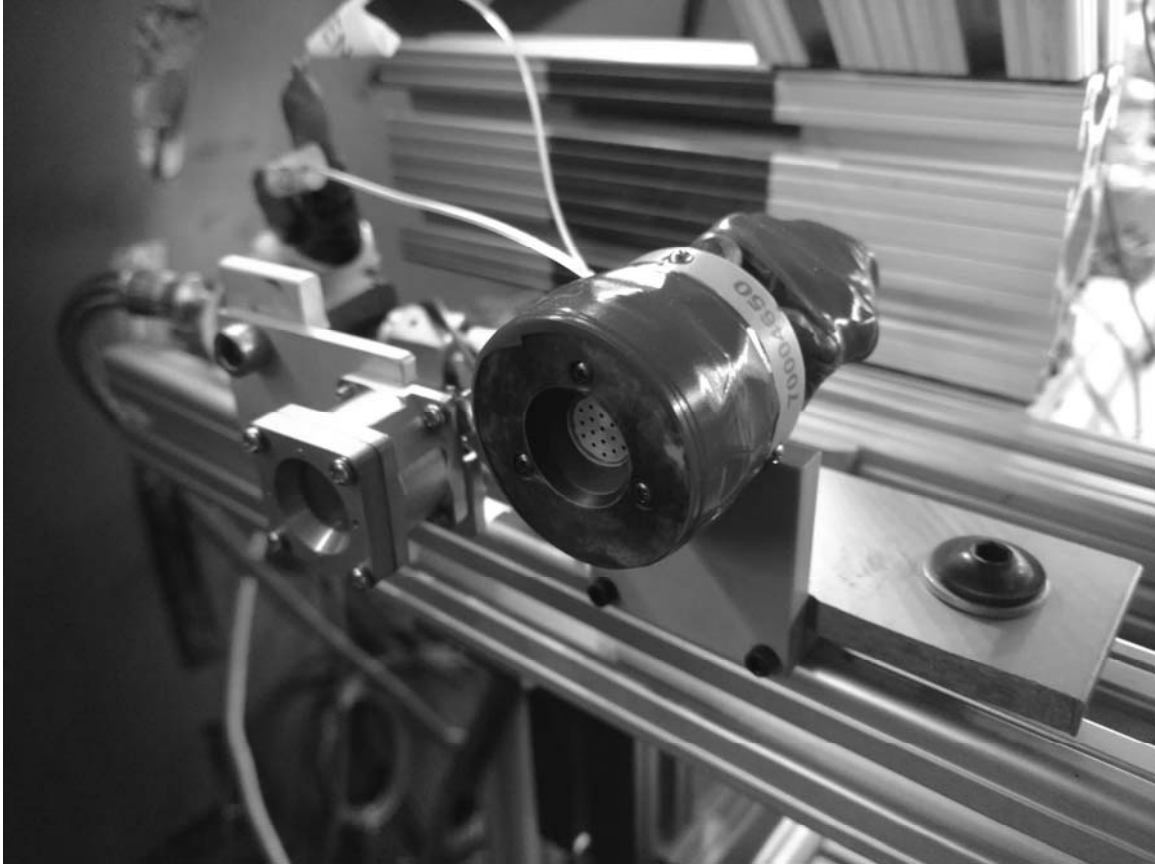
Figure 49. Repaired and Mounted BIT-1 Ion Thruster Wrapped in Silicone Tape
