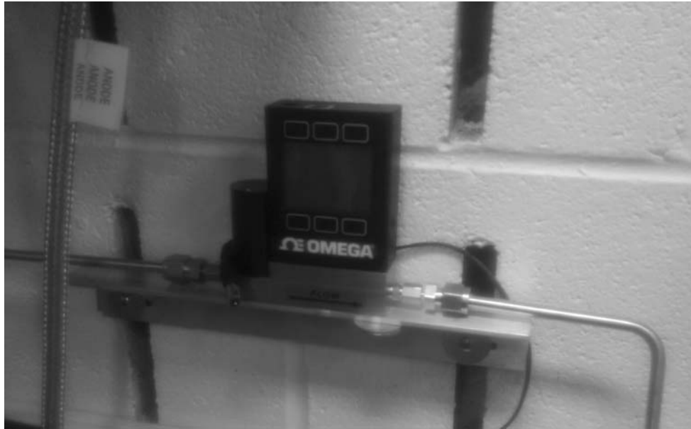
Figure 21. Initial Configuration for FMA-2601A Flow Controller
