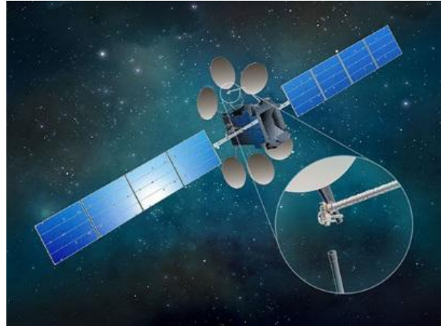
Figure 10: The Dragonfly moves and attaches an antenna to its operational configuration.
