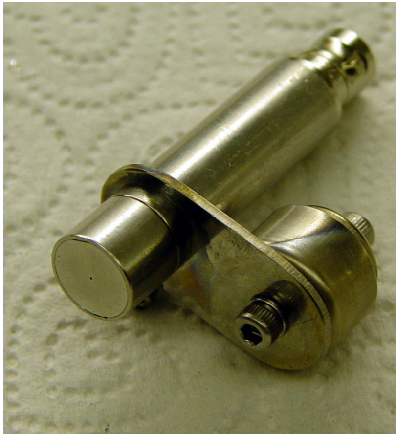
Figure 14. Faraday probe, provided by Plasma Controls [16].
