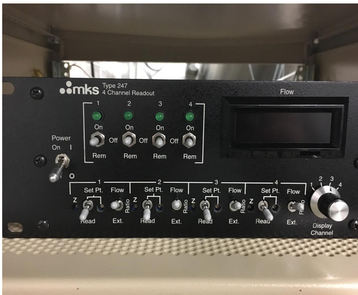
Figure 7. MKS Type 247 flow controller, able to regulate four channels at once.
