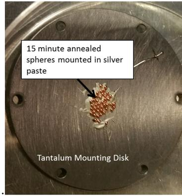
**Figure 3.8.** The picture shows the copper spheres, which were annealed for 15 Min, mounted in silver paste for XPS analysis.
