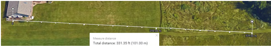
Figure 22. The NI USRP-2921 is positioned at the 0 m marker with RSSI measurements taken along the path of the measurement line.
