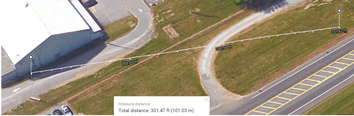
Figure 21. The CENTRON smart meter is positioned at the 0 m marker with RSSI measurements taken along the path of the measurement line.
