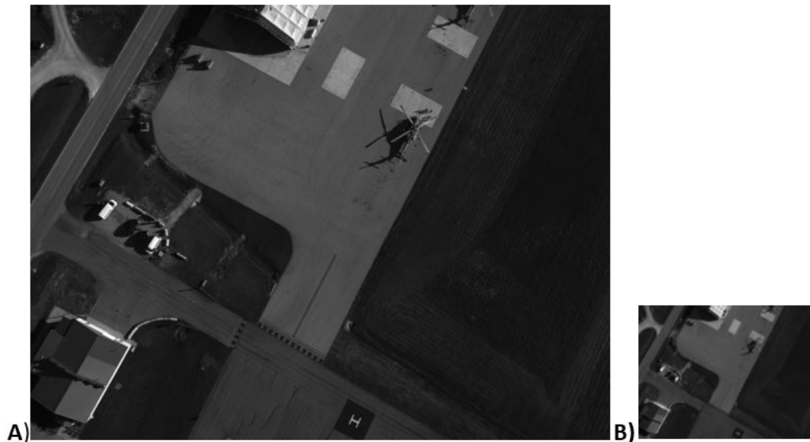
Figure 35. Image A was an image acquired during the flight tests, shown at its full resolution. Image B is the same image, but down-sampled 3 steps to be of comparable resolution to the DigitalGlobe database image.
