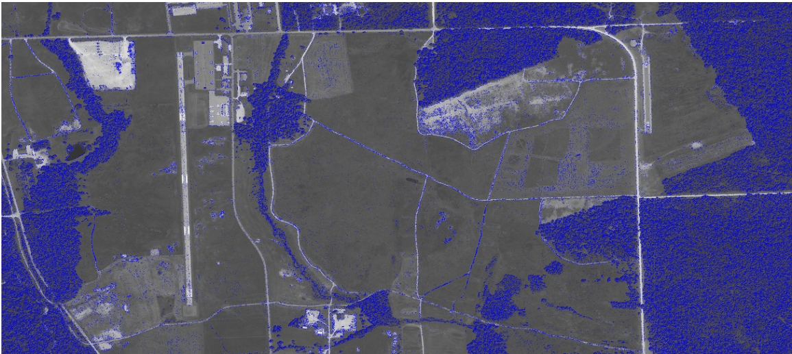
Figure 37. The database variant for the Contrast Threshold set at 0.03 instead of the base of 0.04. Feature locations are shown in blue.
