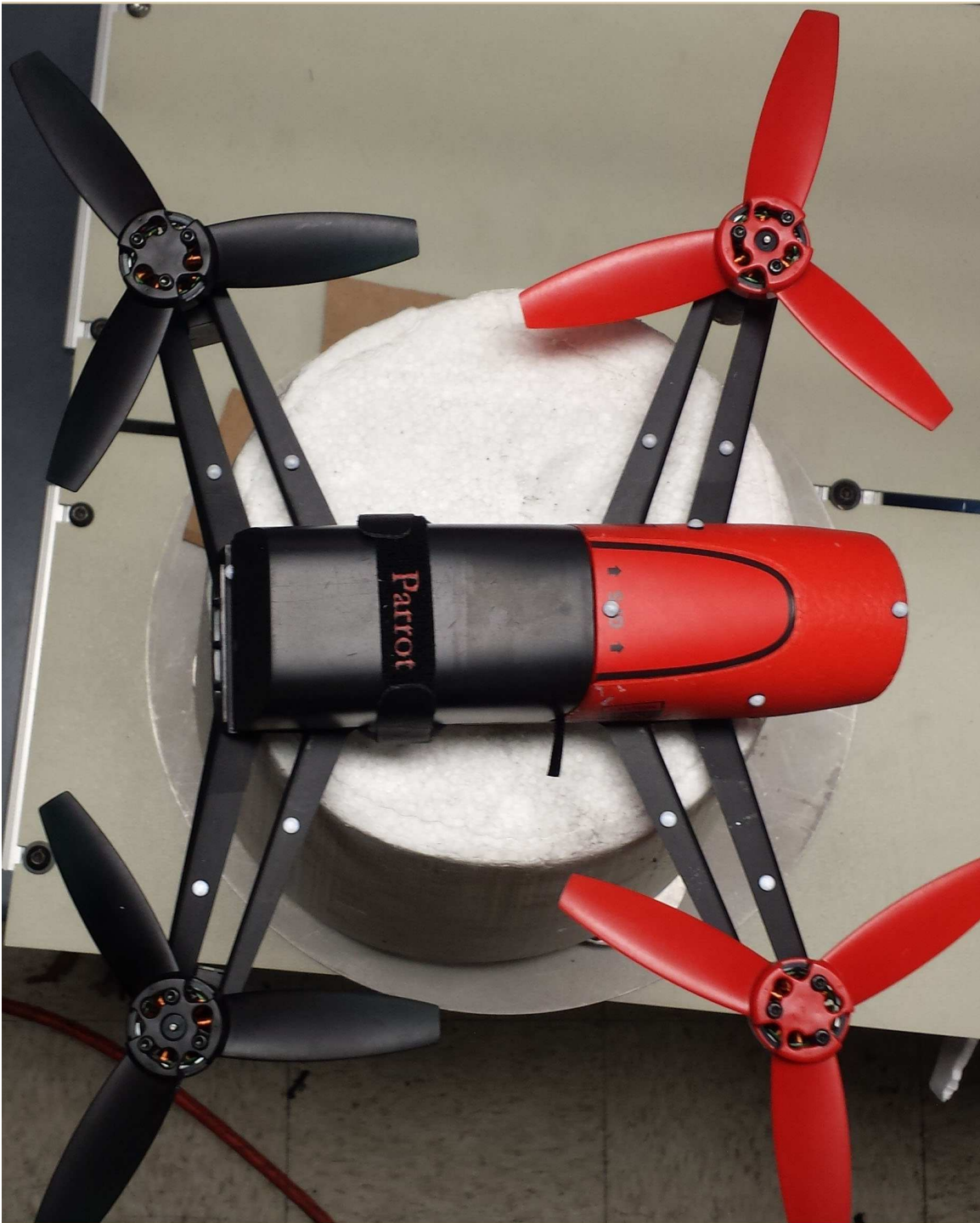
Figure 18. Bebop Reflective Dot Placement: By placing multiple IR reflective dots on the Bebop quadcopter, a unique object was recognized by the Vicon™ system for position and pose data capture.
