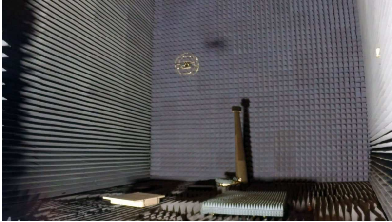
Figure 41. Flying Sphere Encased Quad-Copter: Demonstrated flight capability of a flying Quad-Copter encased in a geodesic sphere with captured radar data.
