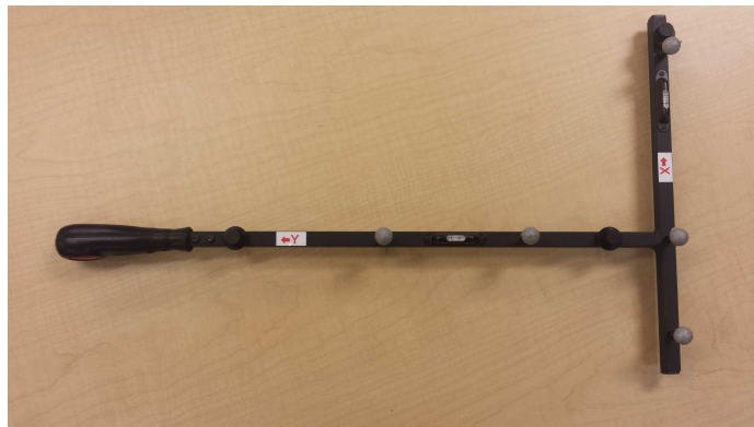
Figure 21. Vicon™ Calibration Wand: Wand for Calibrating the Vicon™ motion capture system.
