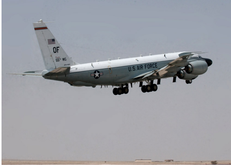
Figure 1. Variant of RC-135 with a cable antenna attached at mid-fuselage to mid-tail. (U.S. Air Force photo/Tech. Sgt. Deborah Davis)
