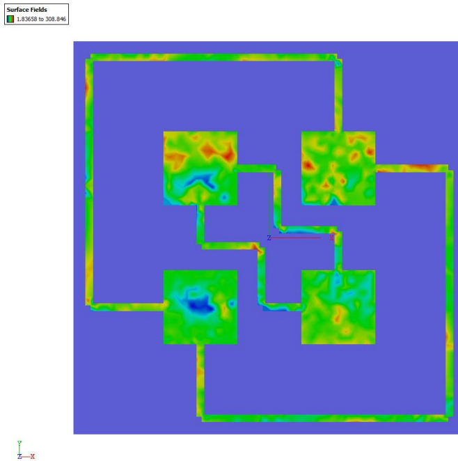
Figure 27. The surface fields at 30 THz \theta = 20^\circ and \phi = 0^\circ excitation of hafnium substrate with 2.5\lambda trace length difference showing phase of electric field.
