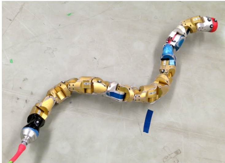
Figure 4.1: The Unified Snake robot, with markers attached for ground-truth motion capture.
