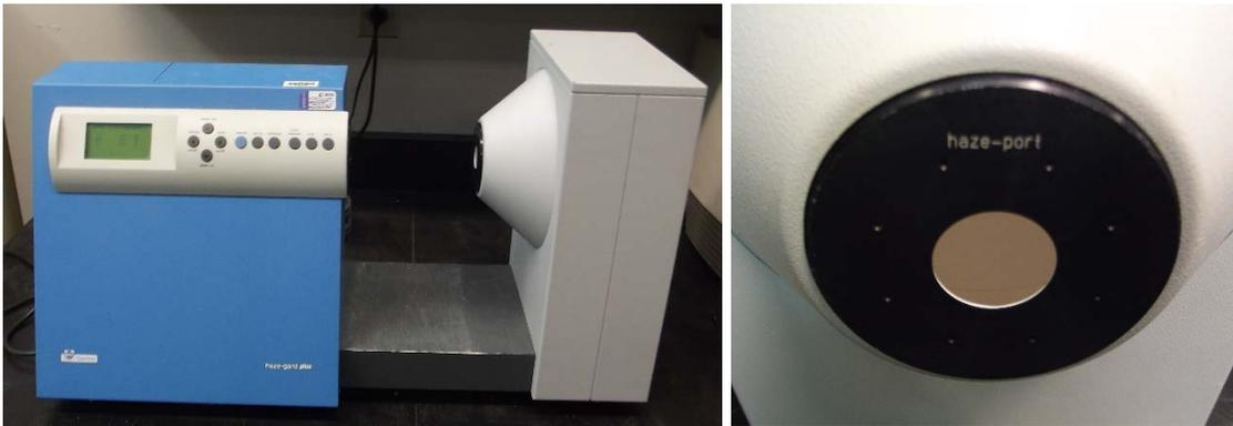
**Fig. 1** haze-gard *plus* (left) with the haze port (right) used to determine the haze in the glass plates
