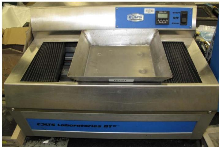
**Fig. 3** Bayer Testing Equipment (BTE) used to abrade the glass plates
