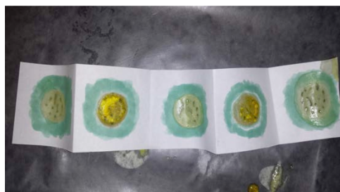
Figure 76: Manually perforated and patterned accordion fold pattern containing hydrogels. Despite patterning a hydrophobic rim around the hydrogel areas.
