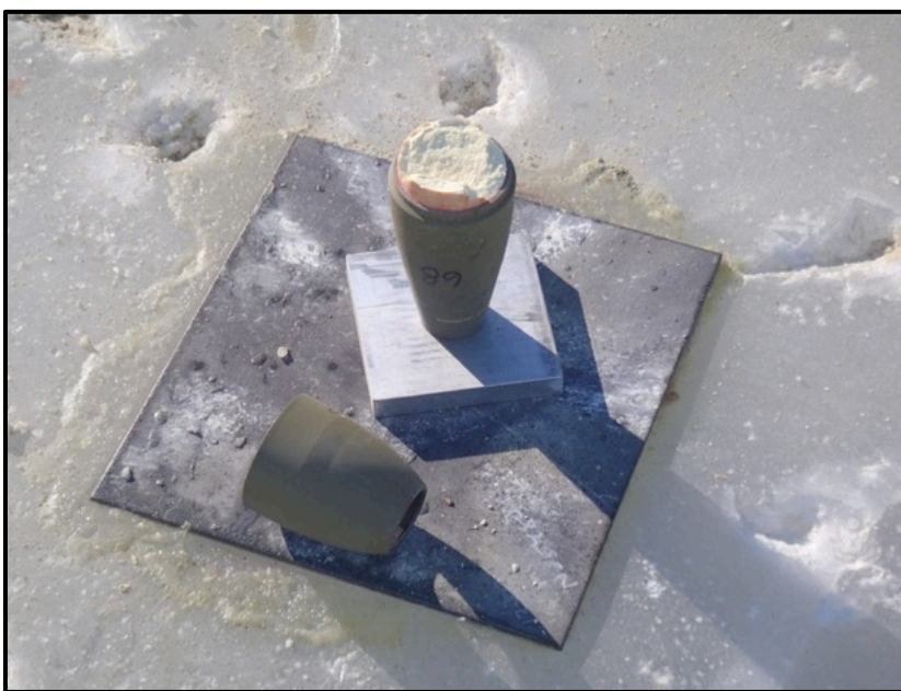
Figure 30. Partial detonation (LO-6) showing filler remaining in body of round
