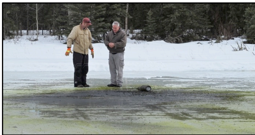
Figure 26. Detonation residues from a M1122 IMX-101 round with a 33-g C4 fuze booster load. Greenish-yellow material on ice surface is dissolved IMX.
