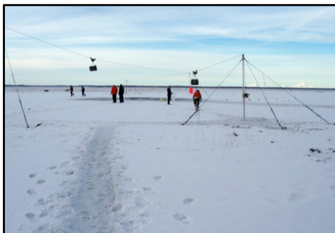
Figure 6. Flyers suspended on cables downwind from C4 detonation point
