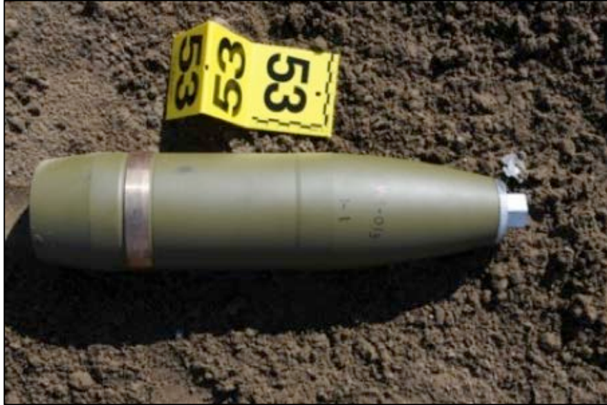
Figure 18. 105-mm IM projectile filled with IMX-104 (without fuse)
