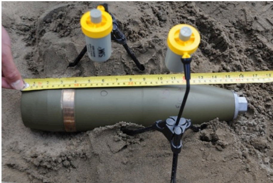
Figure 39. 105-mm IMX-104 round with two SM-EOD 33 at 100-mm stand off distances.
