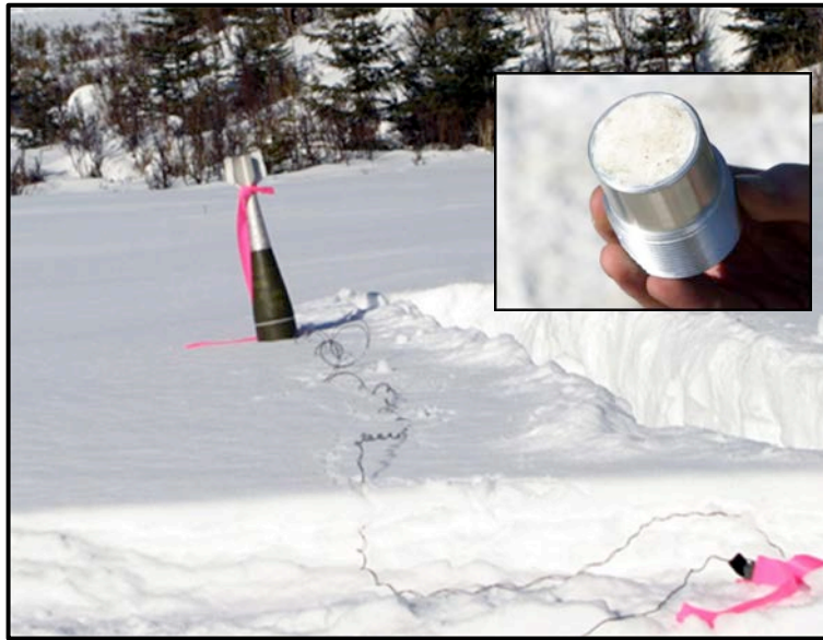
Figure B-2. Set up of detonation point. Fuze adapter shown in inset photo.
