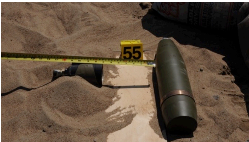
Figure 41. IMX-104 filled 105-mm with one 84-mm shaped-charge at 178 mm stand-off.
