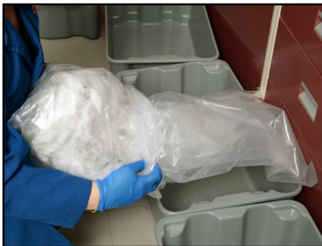
Figure 10. Transferring snow sample to a clean bag prior to melting overnight
