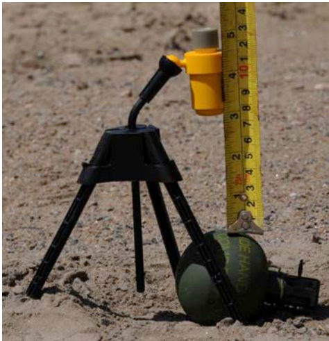
Figure 37. Hand grenade and SM-EOD 20 prior detonation.
