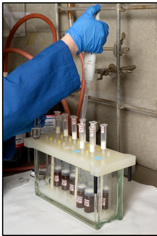
Fig. 14. Measuring the aqueous phase volume Fig. 15. Desorption from Waters Porapak RDX SPE
