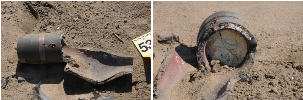
Figure 40. 105-mm filled with IMX-104 after a low-order reaction
