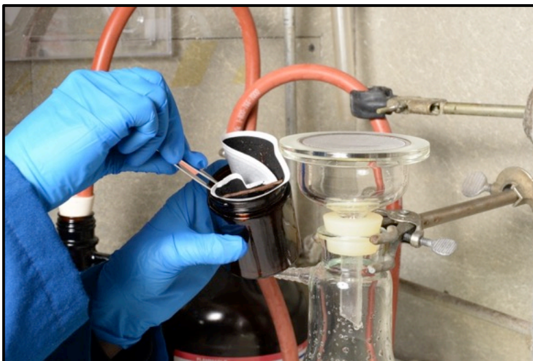
Figure 13. Filters combined and dried in amber glass containers
