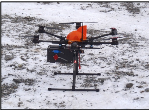
a. UAS on ground. EPA Sensors in black box
