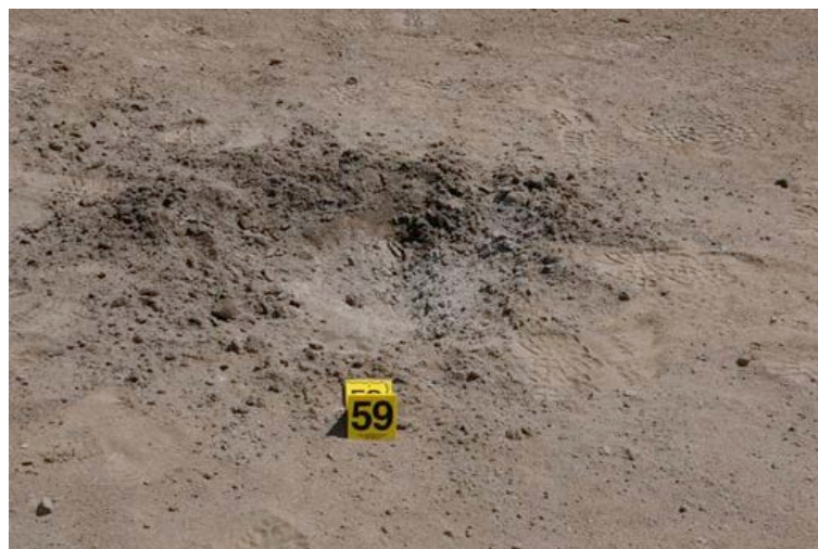
Figure 38. High order crater after BIP of the hand grenade with SM-EOD 20.
