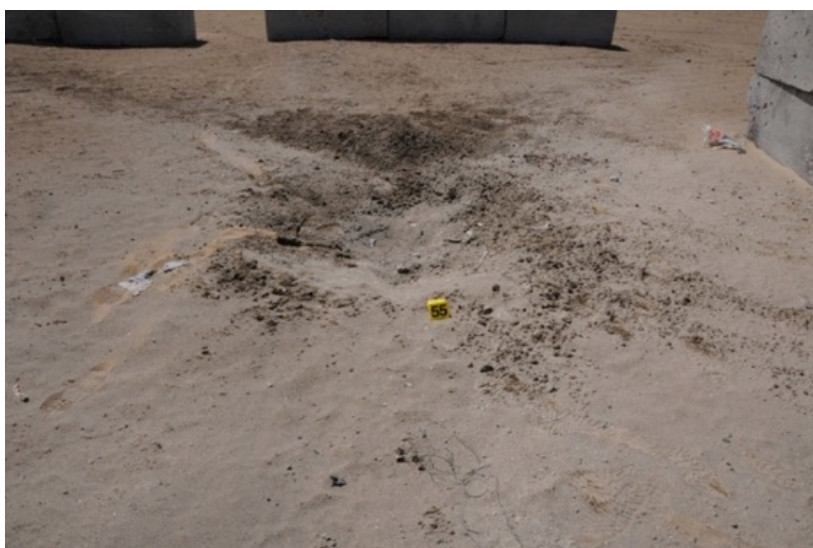
Figure 42. IMX-104 filled 105-mm after a high-order reaction.
