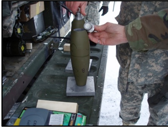
a) Simulator with C4 booster charge
