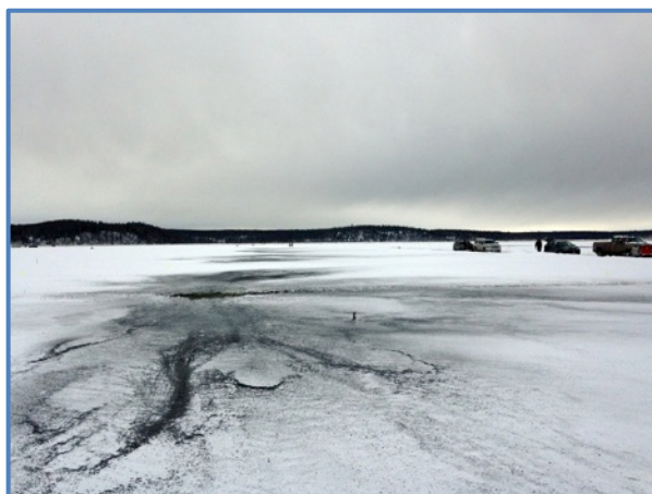
Figure B-5. Residues deposition pattern after detonation
