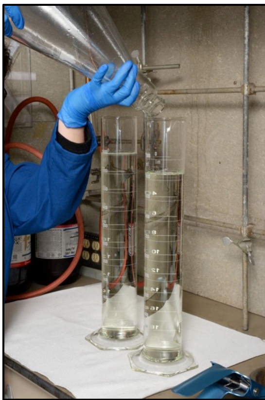
Fig. 14. Measuring the aqueous phase volume Fig. 15. Desorption from Waters Porapak RDX SPE
