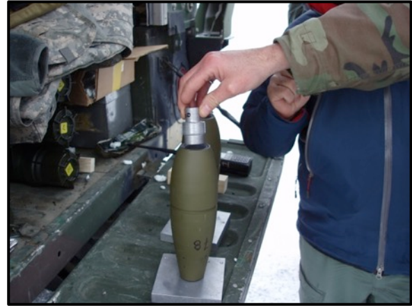
b) Installing simulator in fuze well
