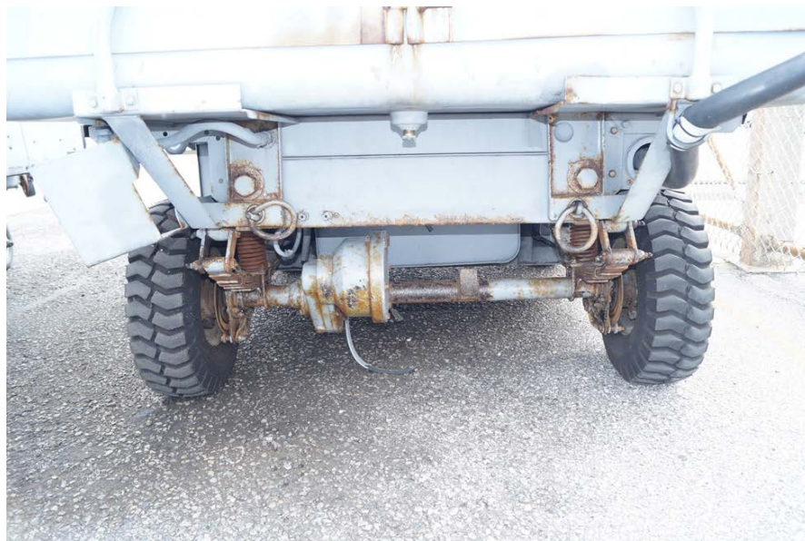
Figure 3 Undercarriage corrosion observed at Kadena AB
