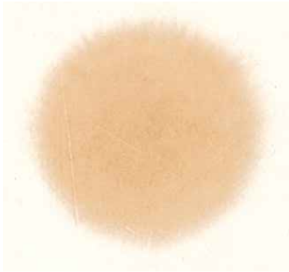
Figure 4.15: Laser beam profile from the 6-stage single pass amplifier on a burn paper.
