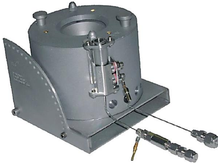
Figure 3-11. An end-Hall ion source showing the typical placement of a filament [68].
