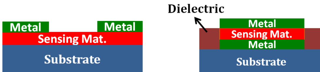
Figure 4-10. The left is the conventional lateral resistance pixel design and the right is the new vertical resistance pixel design [72].
