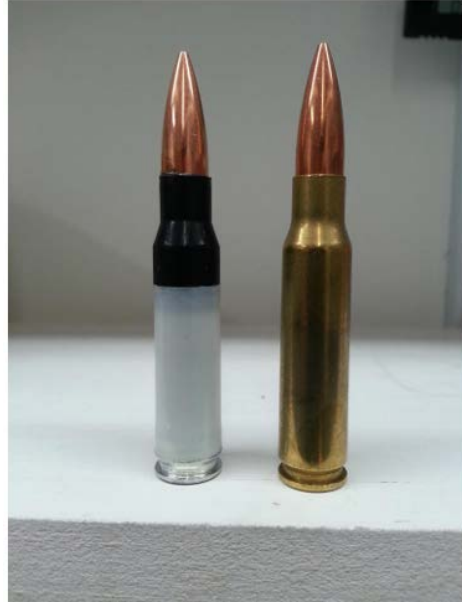
Figure 9. Comparison of Polymer versus Brass-Cased Ammunition. Source: Baker (2014).
