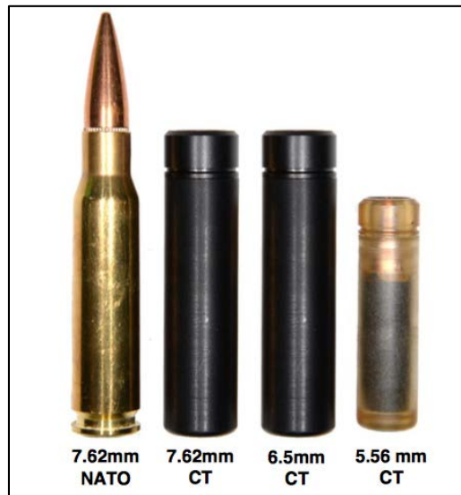
Figure 10. From Left to Right: Traditional Brass-Cased Ammunition versus Case-Telescoped Ammunition. Source: Mizokami (2016).
