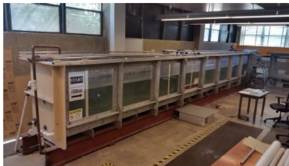
Figure 1.1. NPS Halligan Hall tow tank before wedge installation.
